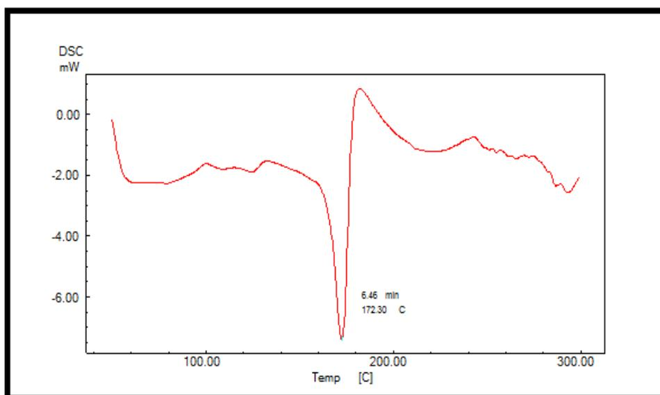
**Figure 4. DSC thermogram of pure candesartan cilexetil**
