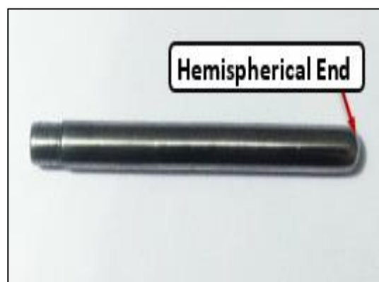
Figure 9: Forming tool used in experimental work
