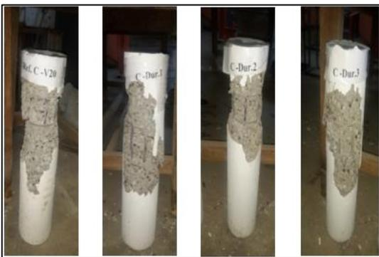
Figure 23: Modes of failure of columns in-group C
