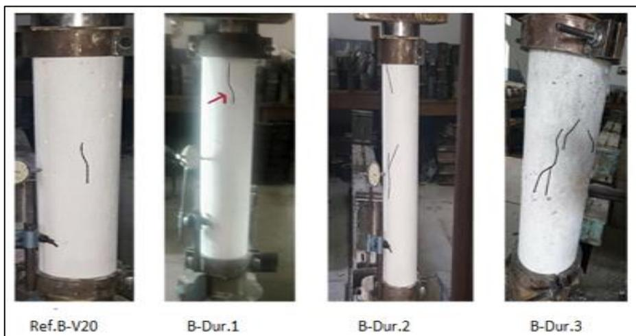
Figure 13: First crack location for each tested specimens
