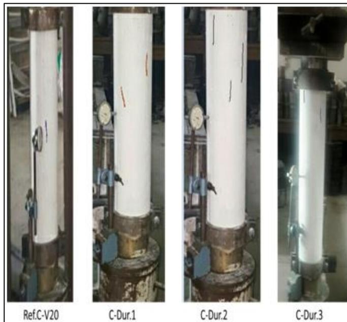
Figure 18: First crack location for main specimens
