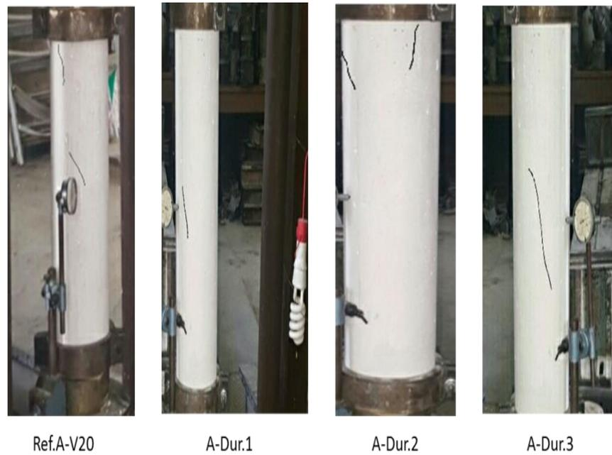
Figure 8: First crack location for each tested specimens
