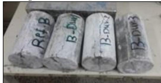
**Figure 15: Concrete cylinders at failure**
