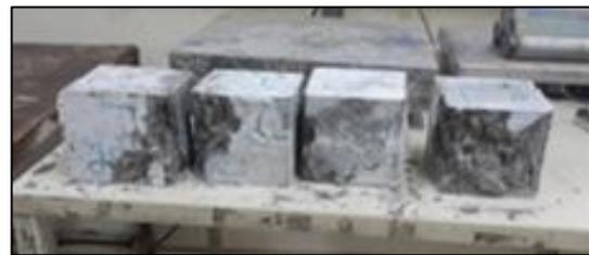
**Figure 14: Concrete cubes at failure**
