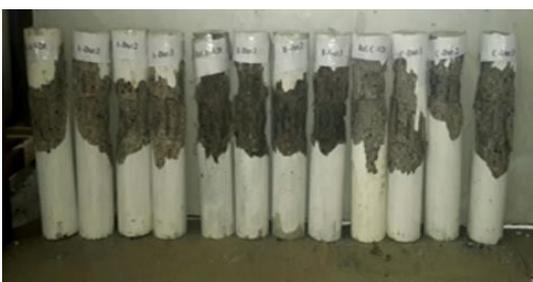
Figure 24: Modes of failure of all columns together
