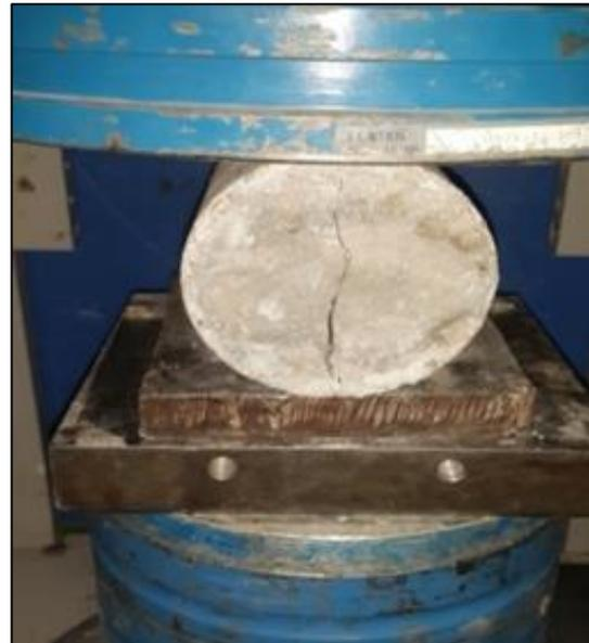
Figure 5: Cylinders splitting tensile test
