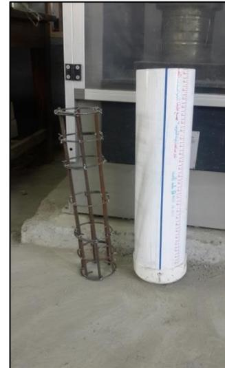
**Figure 2: Molds and reinforcement of tested specimen**
