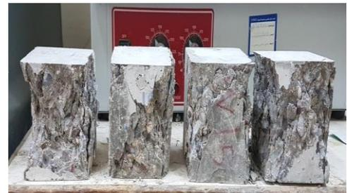
Figure 9: Concrete cubes at failure
