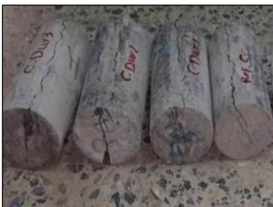
Figure 20: Concrete cylinders at failure
