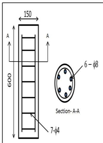
**Figure1: Details of tested specimens**
