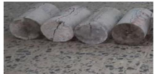
Figure 10: Concrete cylinders at failure
