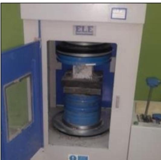
Figure 4: Cubes compressive test
