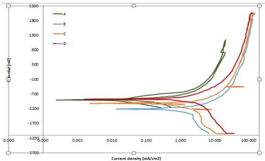
Fig.(10)Electrochemical polarization for all specimens.
