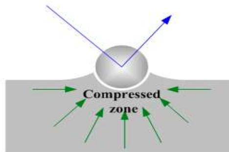
**Fig (1)** A dimple created by shot peening and the resulting compressive zone, Markovina [1991].
