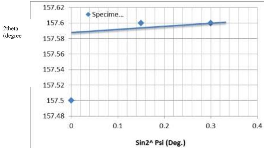
Fig.(5) . photo graph of residual stress for specimen A.
