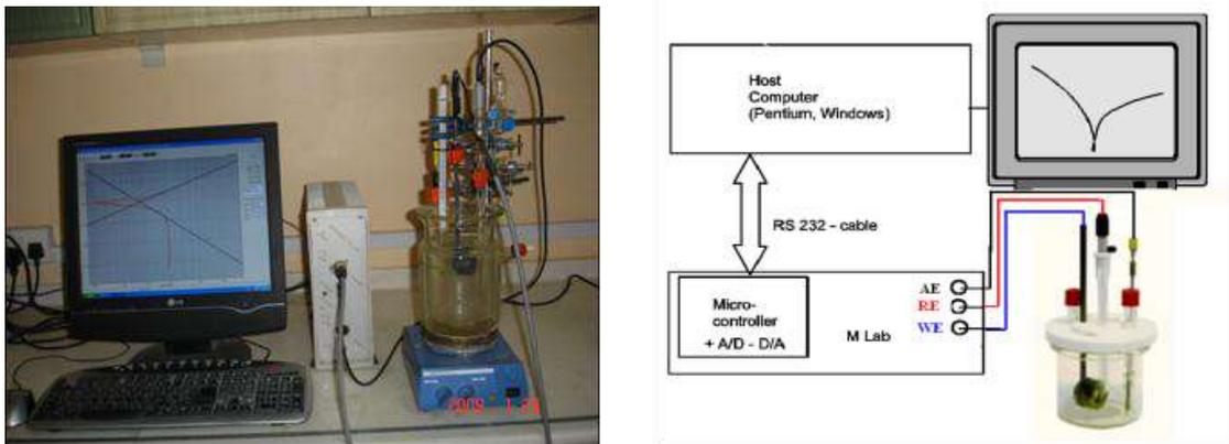
Fig(9)The unit used for electrochemical corrosion.
