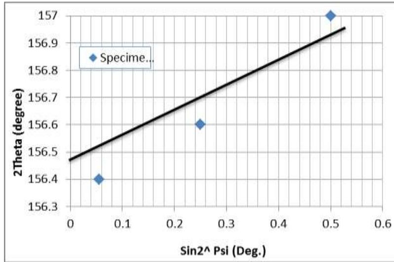
Fig.(8) . photo graph of residual stress for specimen D.
