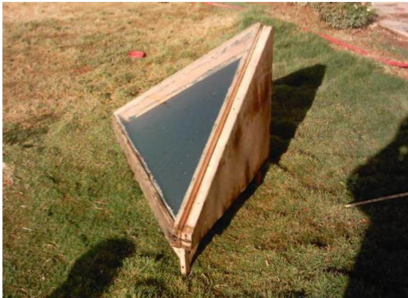
**Figure (2): A photograph of the triangular storage collector.**
