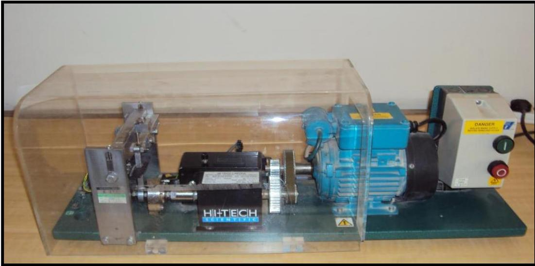
Figure (5): Fatigue test machine.
