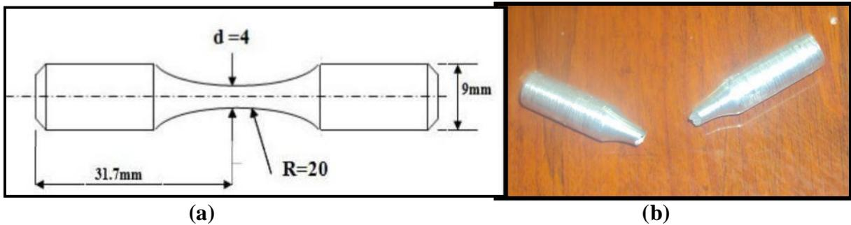
Figure (4): Fatigue test specimen.
