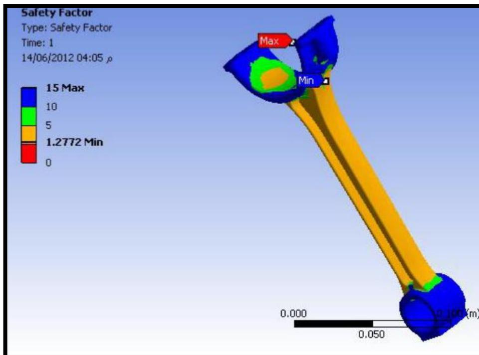
Figure (13): Factor of safety for forged steel.
