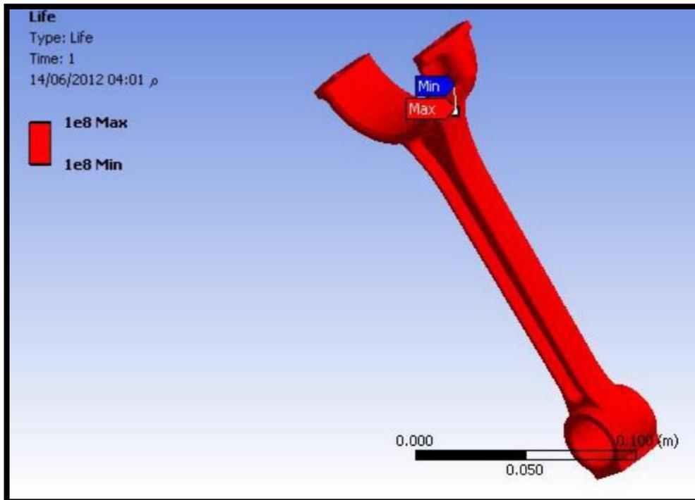
Figure (10): Life for Aluminum Alloy in (cycles).
