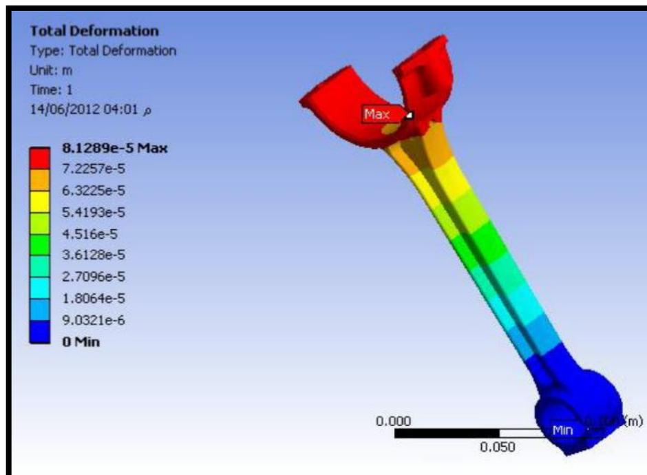
Figure (9): Deformation for Aluminum Alloy in (m).
