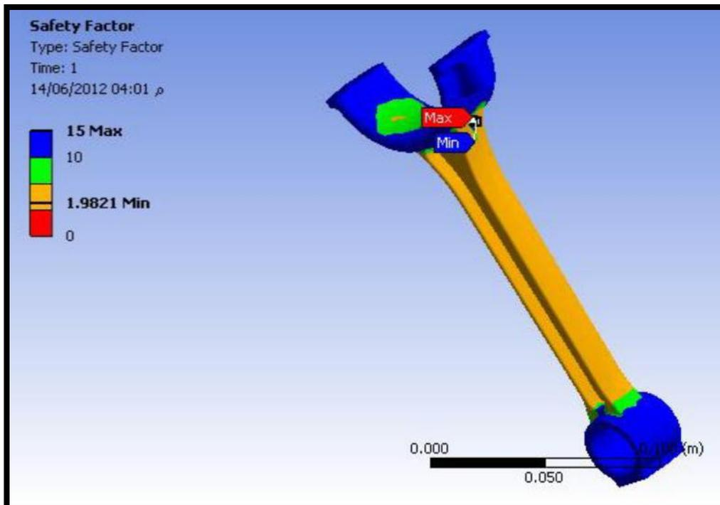
Figure (11): Factor of safety for Aluminum Alloy.
