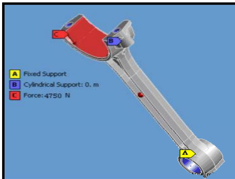
**Figure (7): Loading and supports of connecting rod.**
