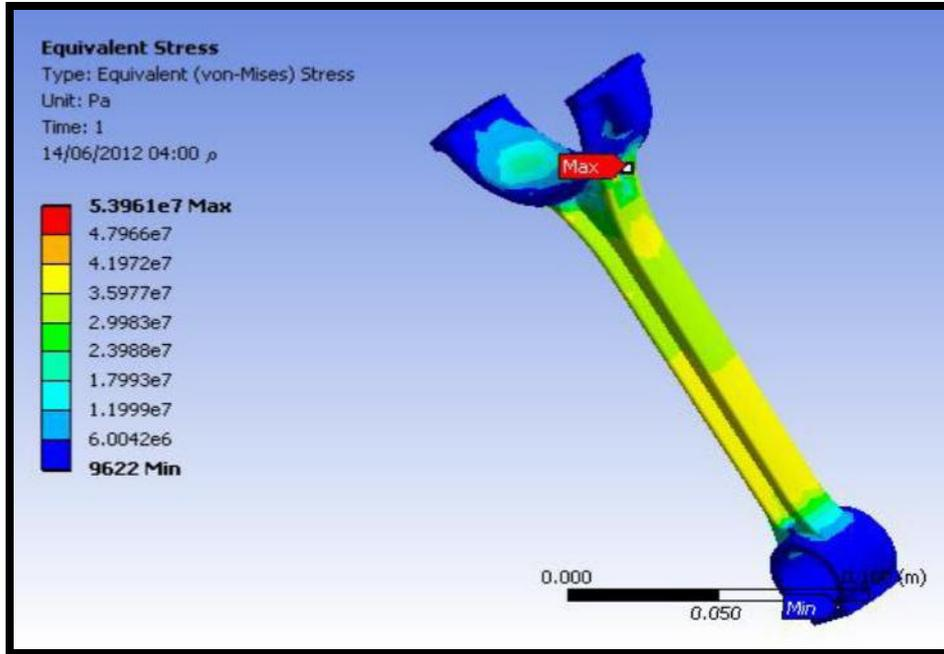
Figure (8): Von – Misses stress for Aluminum Alloy in (Pa).
