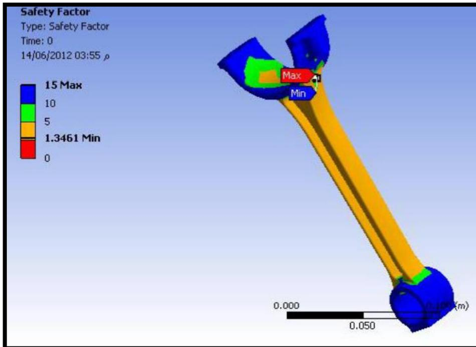
Figure (12): Factor of safety for Titanium Alloy.
