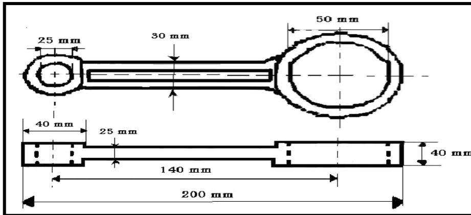
**Figure (3): Dimensions of connecting rod.**
