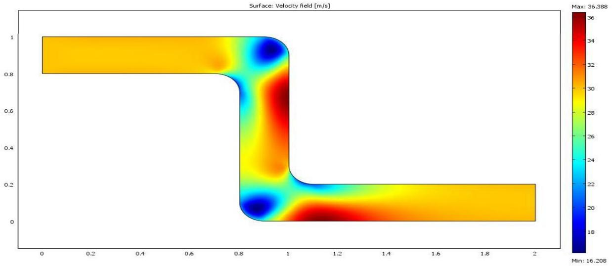
Figure (10): the velocity profile through the channel with double elbow under initial velocity  $u = 30$  m/s
