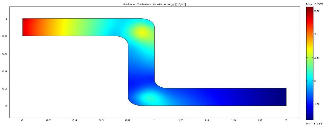
Figure (12): turbulent kinetic energy through the channel with double elbow under inlet velocity  $u = 30$  m/s
