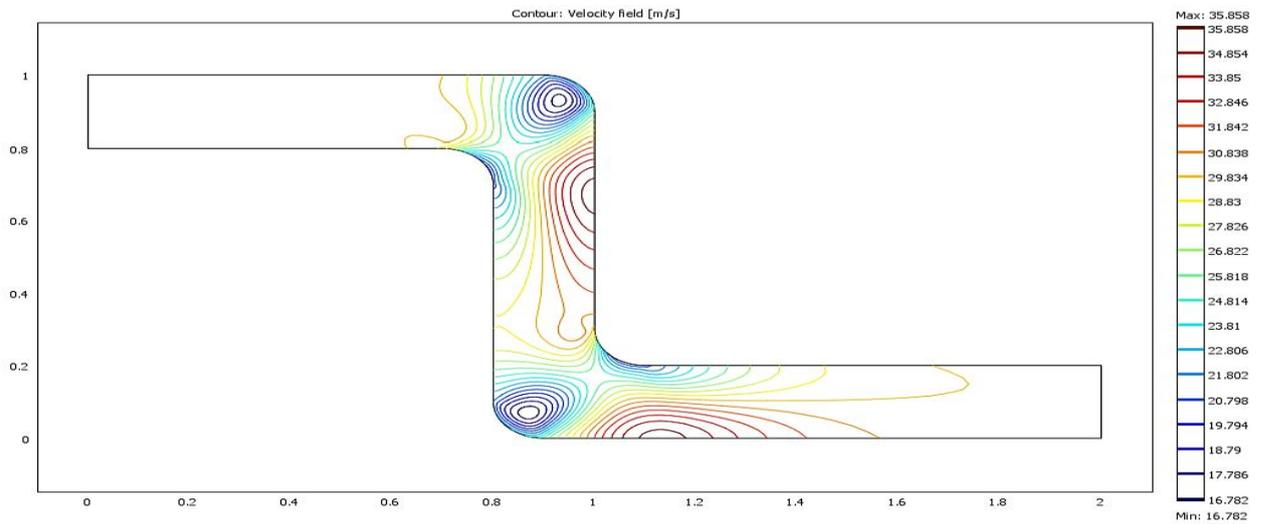
Figure (11): the velocity profile through the channel with double elbow under inlet velocity  $u = 30$  m/s
