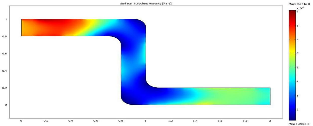
Figure (8): turbulent viscosity through the channel with double elbow under inlet velocity  $u = 20$  m/s
