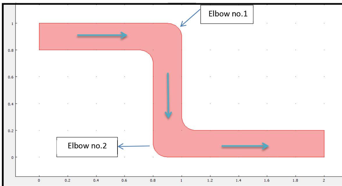
**Figure (2): the geometrical shape of the channel with double elbow**
