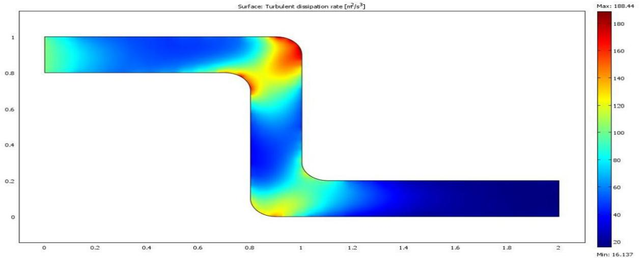
Figure (13): turbulent dissipation rate through the channel with double elbow under inlet velocity  $u = 30$  m/s
