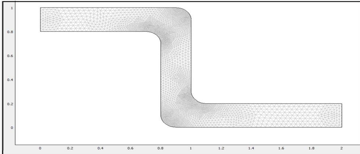
Figure (3): the physical domain of channel with mesh divisions
