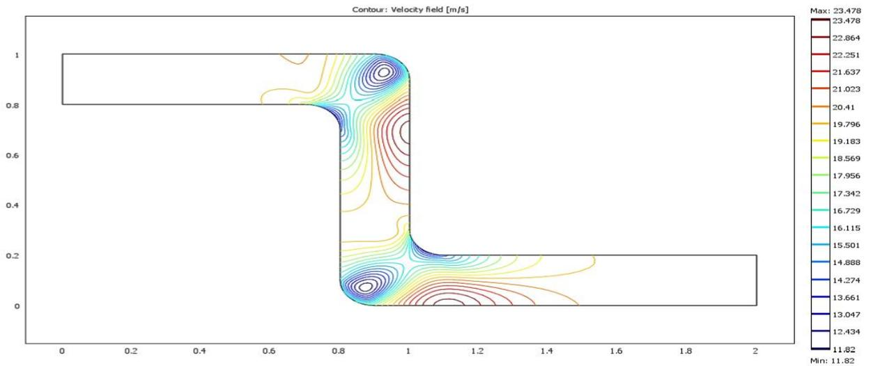
Figure (5): the velocity coontours through the channel with double elbow under inlet velocity  $u = 20$  m/s
