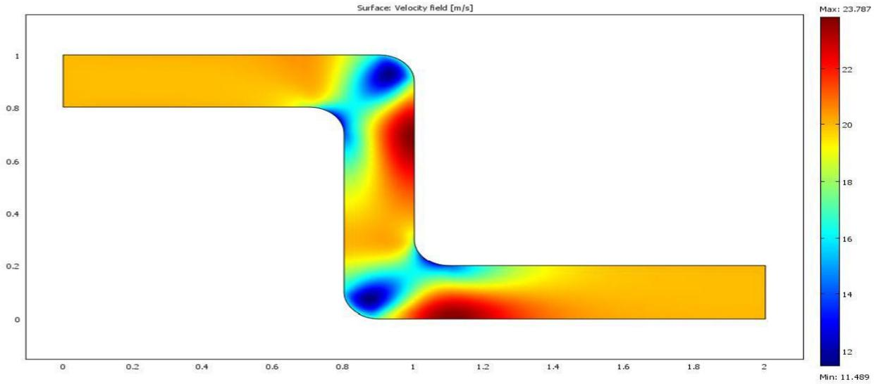
Figure (4): the velocity profile through the channel with double elbow under initial velocity  $u = 20$  m/s
