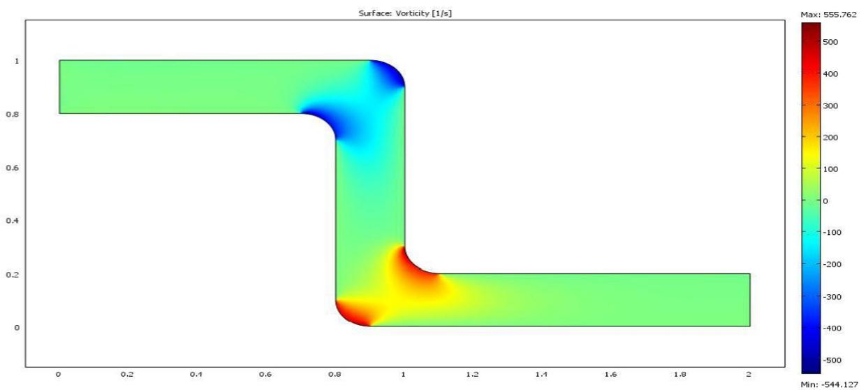
Figure (15): the vortices through the channel with double elbow under inlet velocity  $u = 30$  m/s
