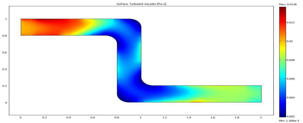
Figure (14): turbulent viscosity through the channel with double elbow under initial velocity  $u = 30$  m/s
