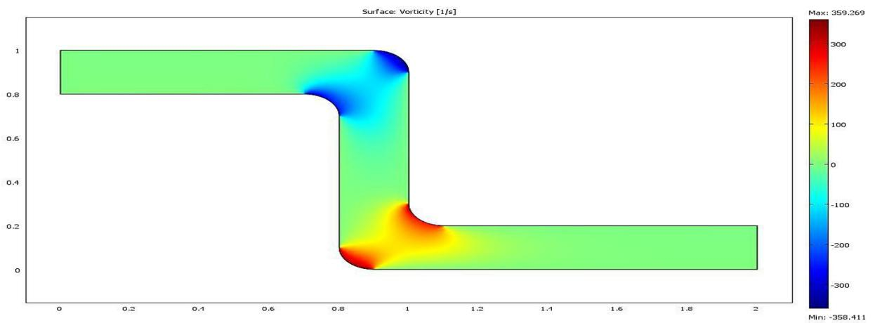
Figure (9): the vortices through the channel with double elbow under inlet velocity  $u = 20$  m/s
