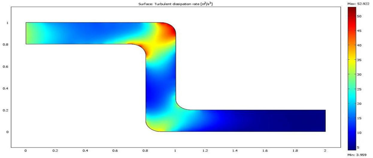
Figure (7): turbulent dissipation rate through the channel with double elbow under inlet velocity  $u = 20$  m/s
