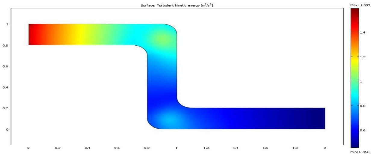
Figure (6): turbulent kinetic energy through the channel with double elbow under inlet velocity  $u = 20$  m/s
