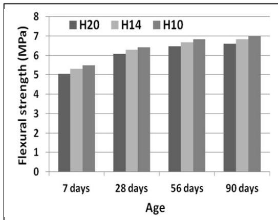
Figure (5): Development of flexural strength for different mixes of HSC
