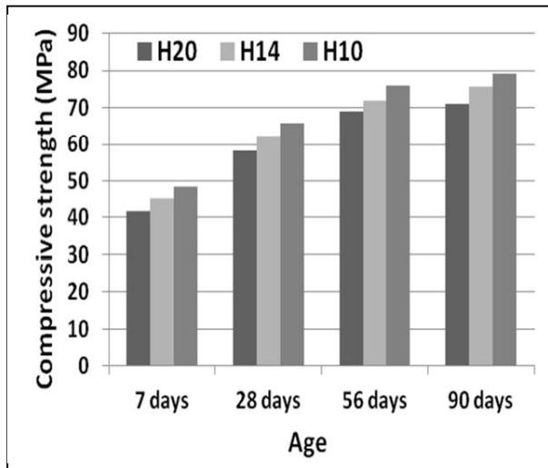
Figure (1): Development of compressive strength ( $f_{cu}$ ) for different mixes of HSC
