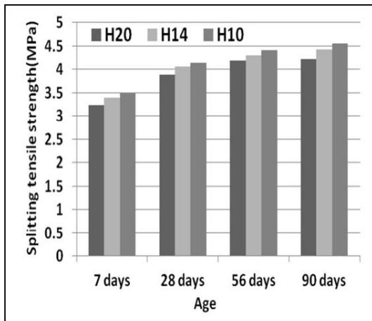
Figure (3): Development of splitting tensile strength for different mixes of HSC
