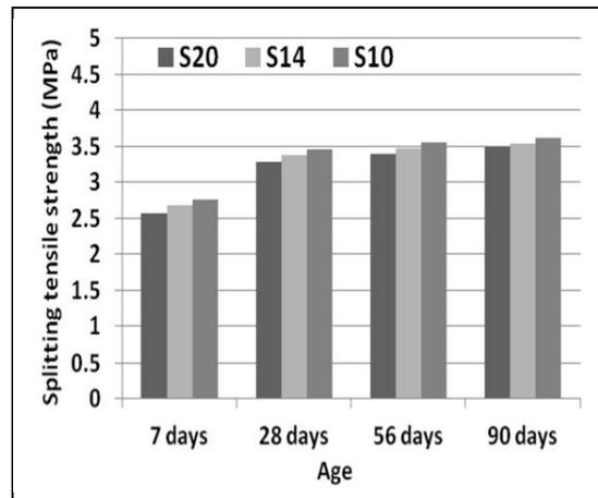
Figure (4): Development of splitting tensile strength for different mixes of SCC
