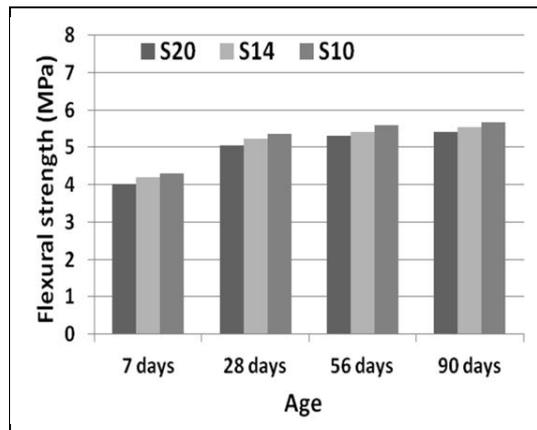
Figure (6): Development of flexural strength for different mixes of SCC
