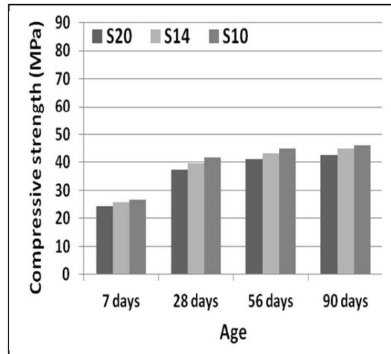
Figure (2): Development of compressive strength ( $f_{cu}$ ) for different mixes of SCC
