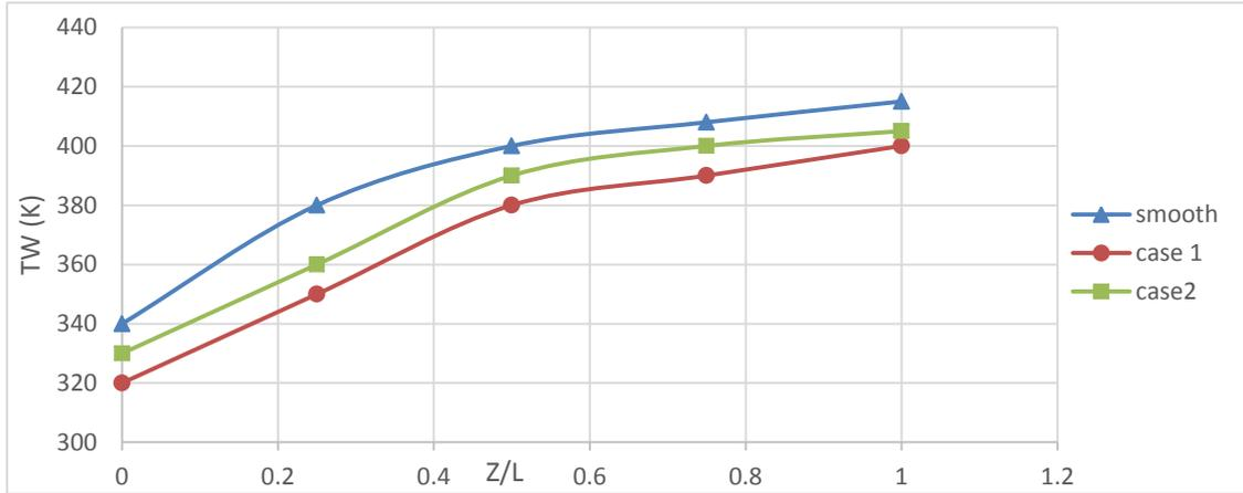
**Figure (7) Temperature distribution along the channel inner wall**
