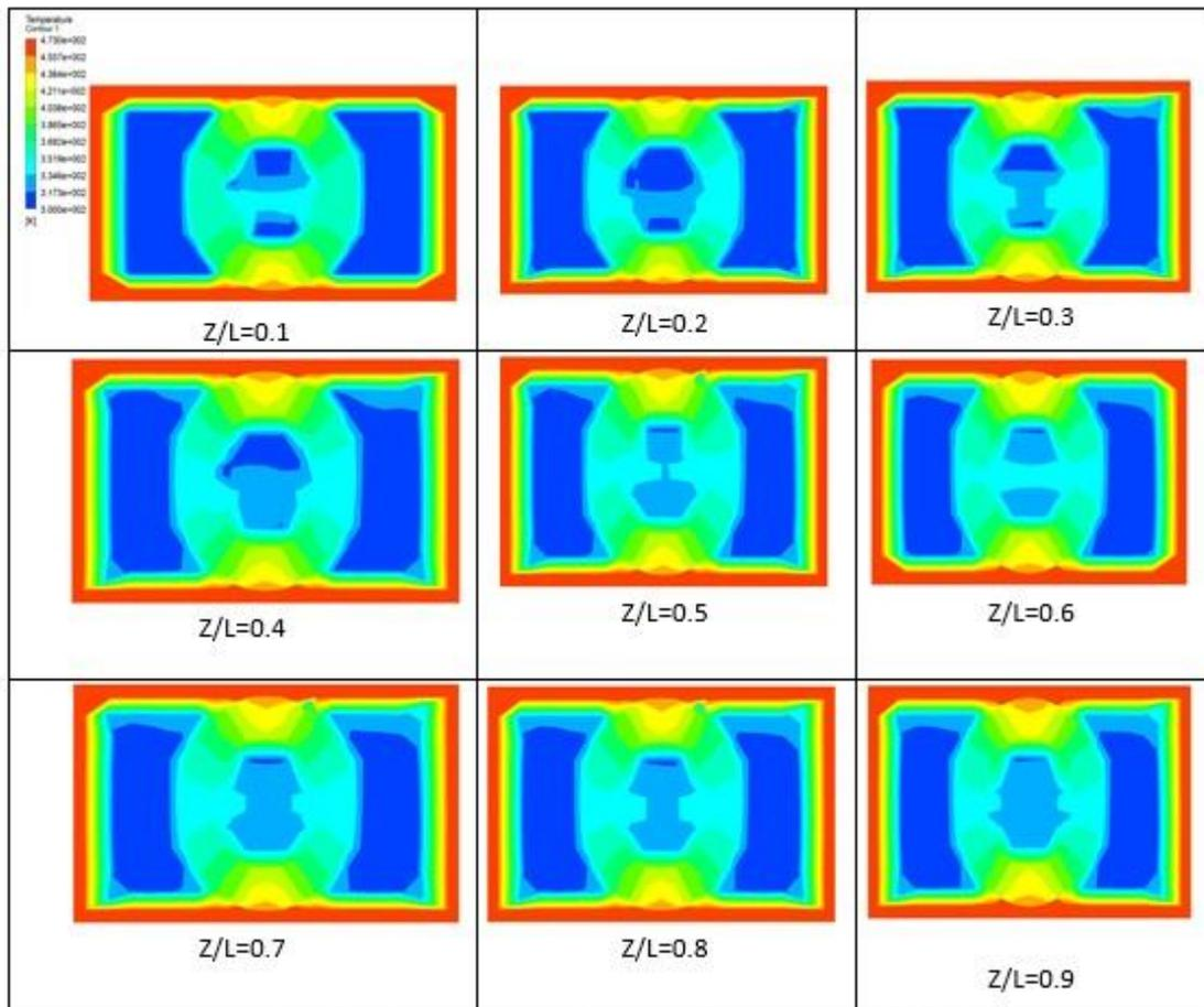
**Figure (13) contour of temperature distribution at each rib for case 1**
