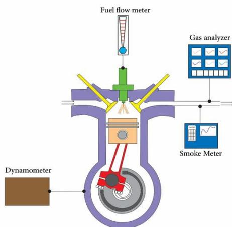
Figure 1: Schematic of the rig
