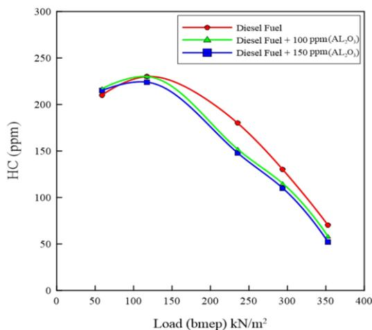
**Figure 7: The HC at different loads for three types of fuels**
