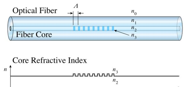
Figure 1: Fiber Bragg Grating structure
