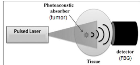
Figure 3: Photoacoustic principle
