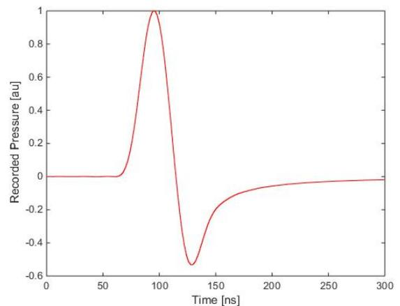
Figure 5: Photoacoustic signal
