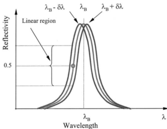
Figure 2: wavelengths Spectrum Shift in the FBG
