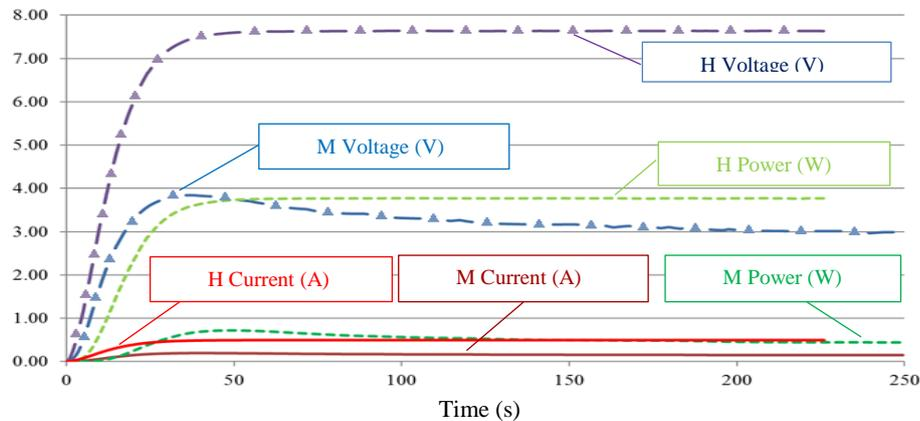
**Figure 10:** PID control setting time of the anode voltage, drain current and consumed power for both levels of soil moisture (M and H levels).
