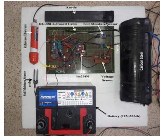
**Figure 2:** The built ICCP system components.
