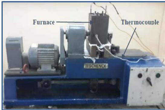
Figure 3: Furnace attached to fatigue machine.
