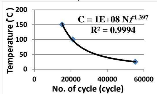
**Figure 9:** S-N curve equation at constant stress  $\sigma = 275$  MPa.
