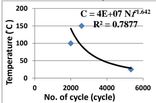
**Figure 8:** S-N curve equation at constant stress  $\sigma = 350$  MPa.
