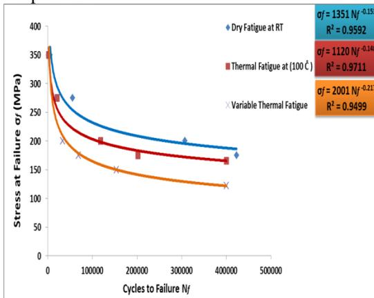
**Figure 5:** S-N Curve for Three Fatigue Test Conditions.
