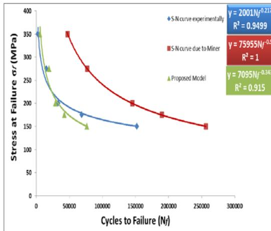
**Figure 6.** Comparison between the Experimental, Miner and Proposed model S-N Curve.
