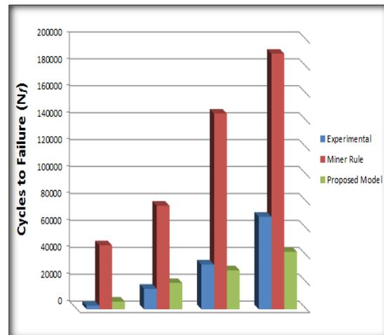
**Figure 7.** Comparison between Three Methods of Prediction Experimental, Miner Rule and Proposed Model for Fatigue Lives under Thermal Variable Temperature of 2017-T4 Aluminum Alloy
