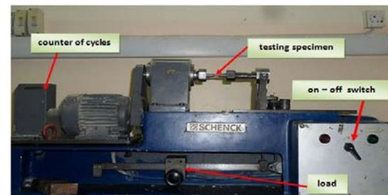
Figure 2: Fatigue testing apparatus.
