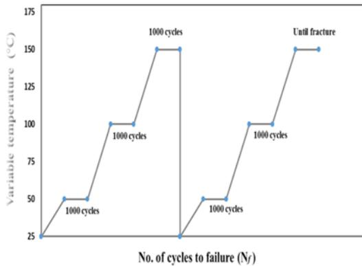
**Figure 4:** Variable Temperature Constant Stress Amplitude Fatigue Test Diagram.
