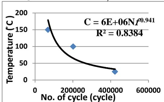
**Figure 10:** S-N curve equation at constant stress  $\sigma = 175$  MPa.
