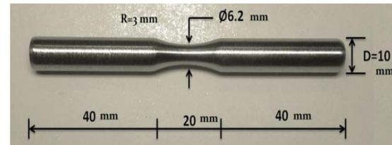
Figure 1: Fatigue test specimen according to the ASTM81-8 standard specification. [9]
