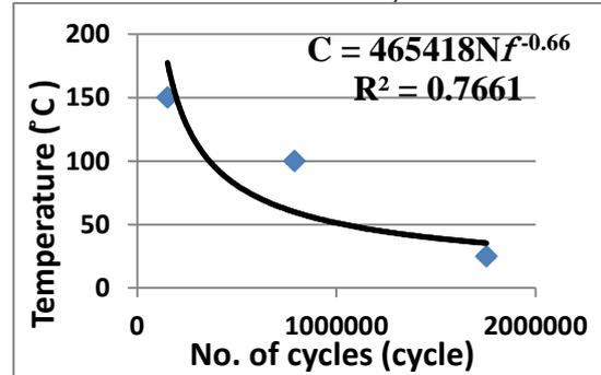
**Figure 11:** S-N curve equation at constant stress  $\sigma = 150$  MPa.
