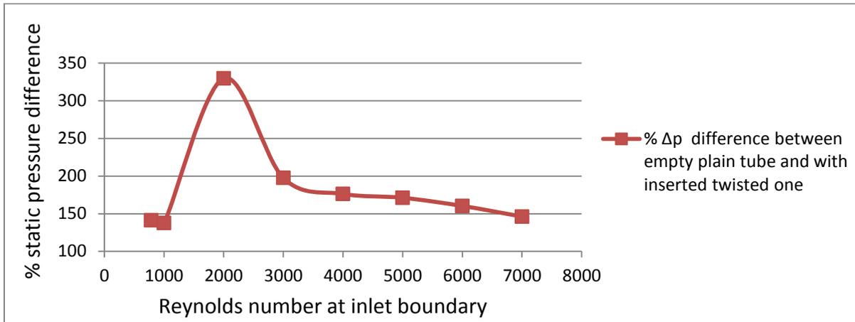
Figure 5. Variation of percentage static pressure difference increase with inlet Reynolds numbers for plain tube inserted with twisted tape over empty plain tube.
