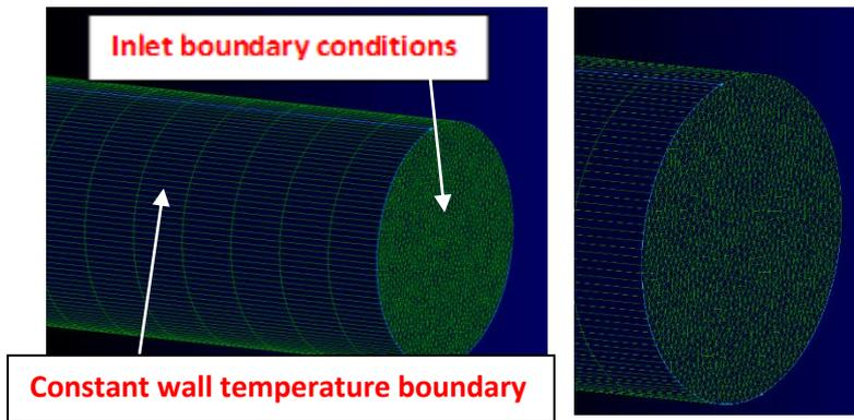
Figure 2. (b) Hybrid mesh of plain empty tube.
