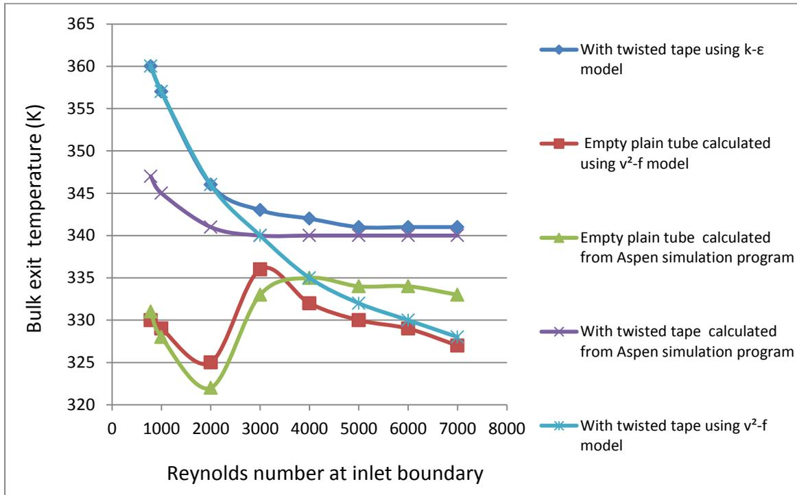
**Figure 3.** Bulk exit temperature of crude oil API 28 from empty plain tube and plain tube with inserted with twisted tape.
