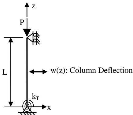
**Figure 2:** Pinned ends column with a torsional spring at the lower support (upper column)
