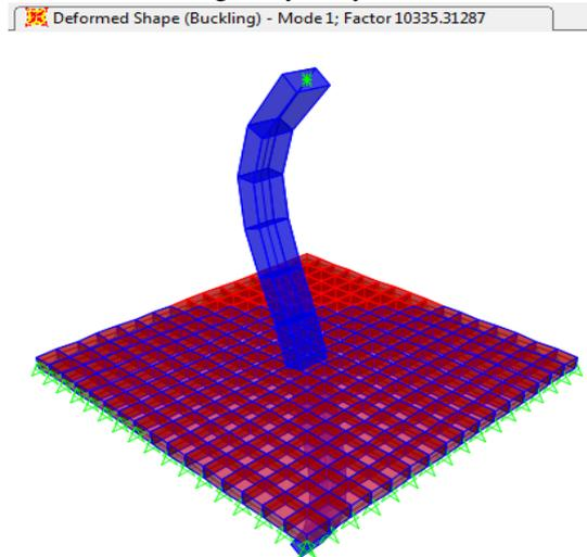
Figure 5: A 3-D finite element model in SAP2000: second buckling analysis
