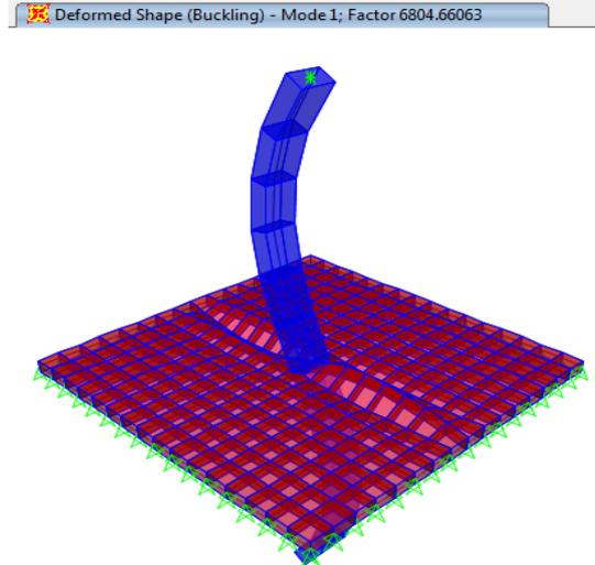
Figure 4: A 3-D finite element model in SAP2000: first buckling analysis
