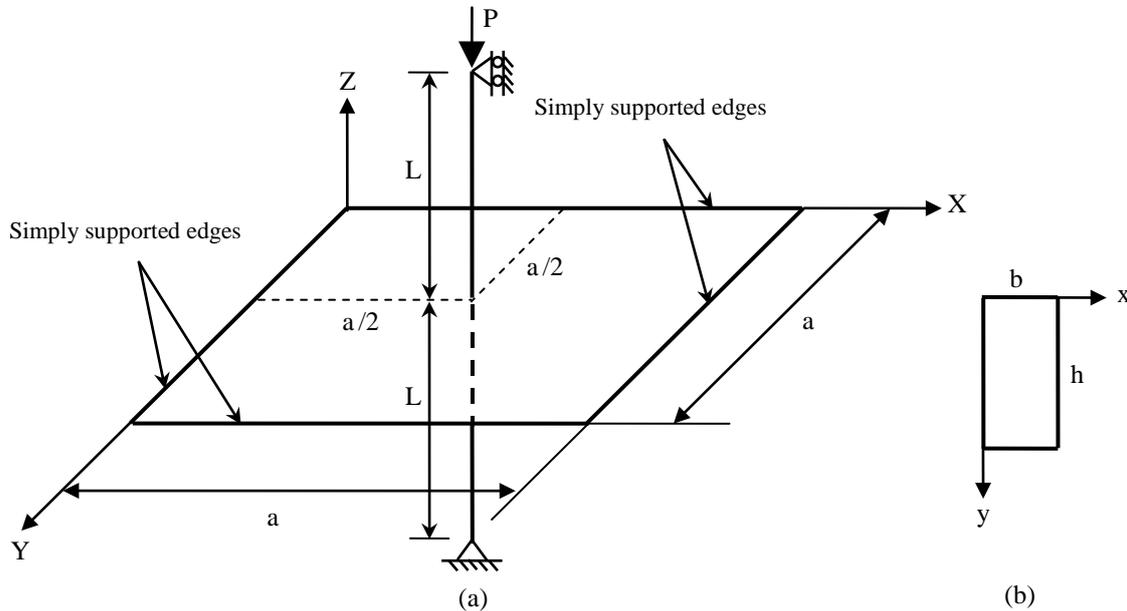
**Figure 1:** (a) Pinned ends column bolted to a simply supported plate (b) Column Cross-section
