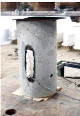
a) 2 strain gauges for tested cylinder
