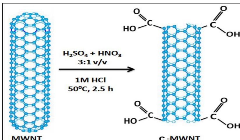
Fig. (2): Carboxylation of MWNTs [15]
