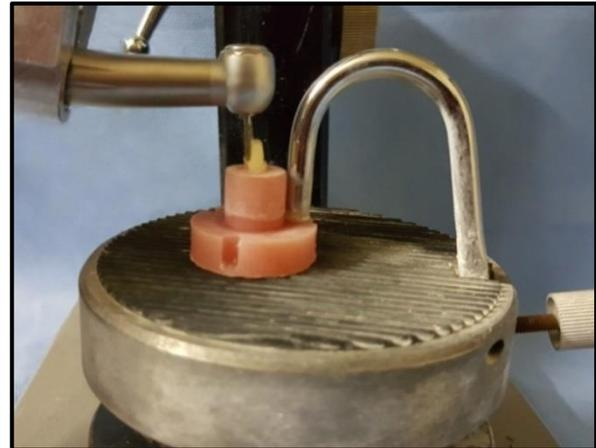
Figure 1: Tooth preparation using a modified dental surveyor.
