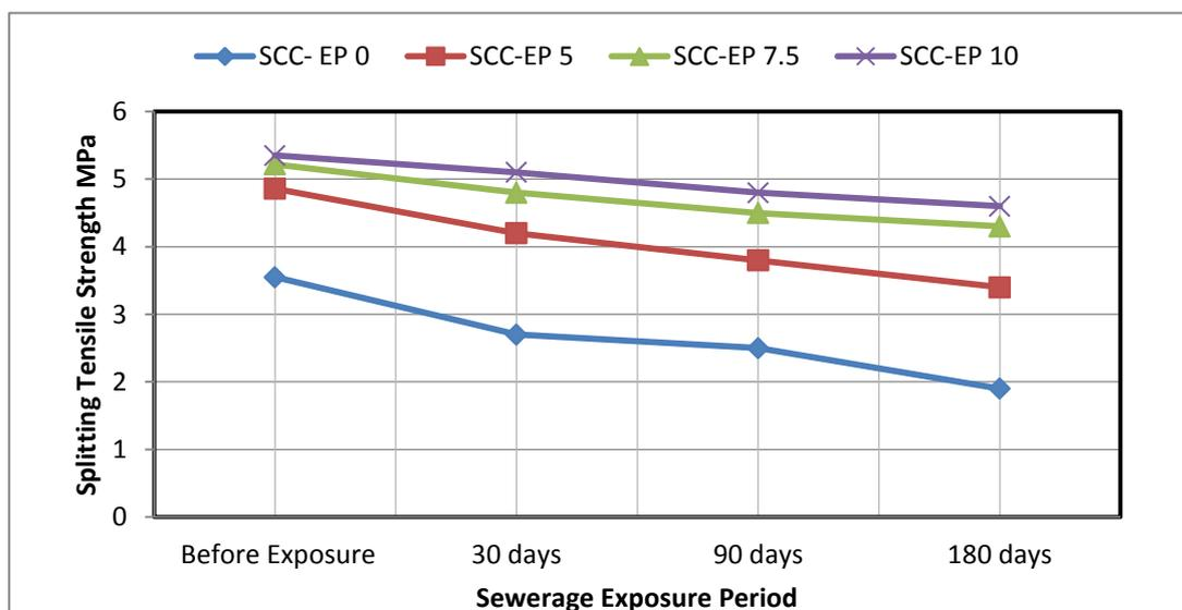
Fig. 3 : Splitting tensile strength of epoxy modified SCC mixes exposed to sewerage
