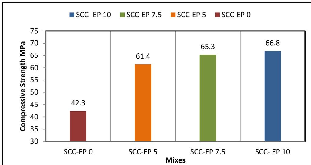
Fig. 1 Compressive strength of various types of SCC-EP at 28 days water curing
