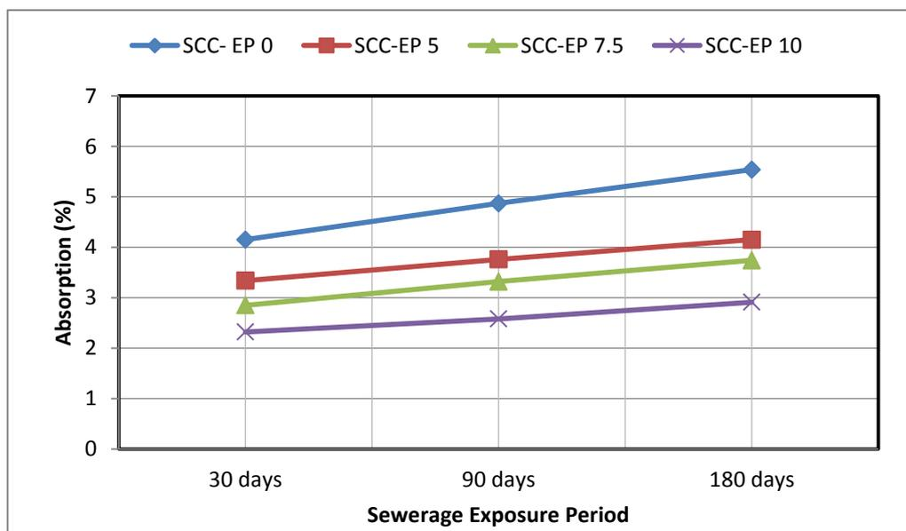
Fig. 5 : Absorption of epoxy modified SCC mixes exposed to sewerage
