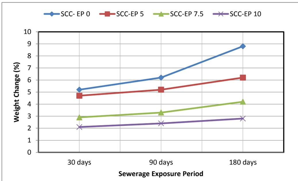
Fig. 4 : Weight change of epoxy modified SCC mixes exposed to sewerage
