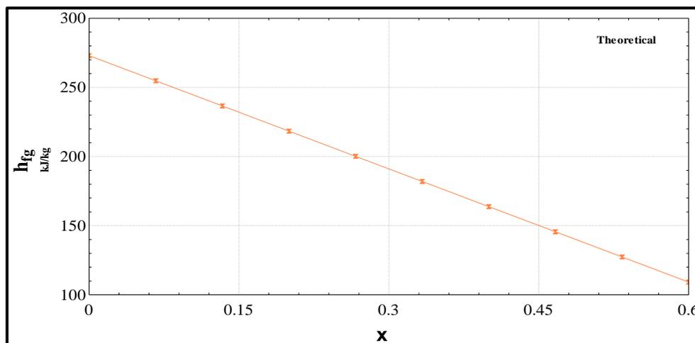
Figure (8) Refrigerating latent heat vs. amount of refrigerant flashing gas
