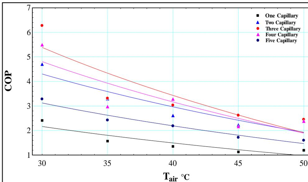
Figure (11) COP vs. ambient air temperature
