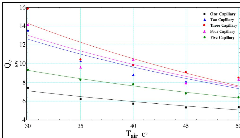
Figure (6) Condenser heat rejection vs. ambient air temperature
