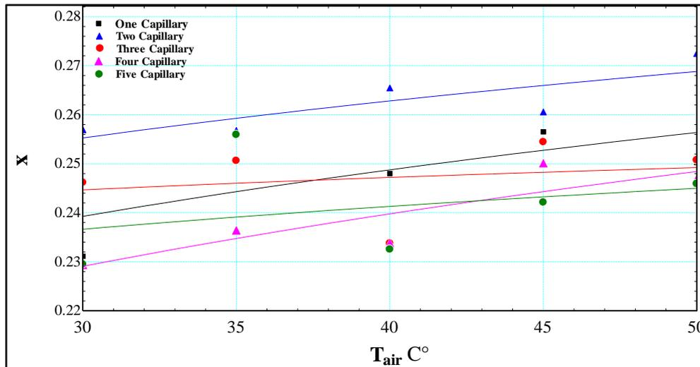
Figure (5) Flashing gas quality vs. capillary tube number
