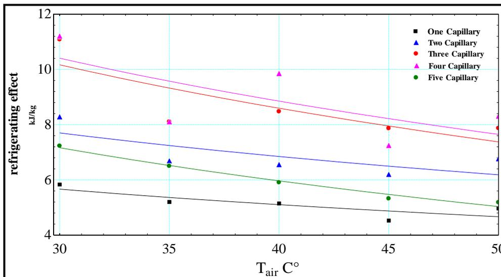
Figure (7) Refrigerating effect vs. ambient air temperature
