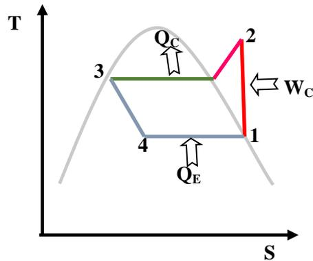
Figure (1) Vapor compression cycle on T-S diagram
