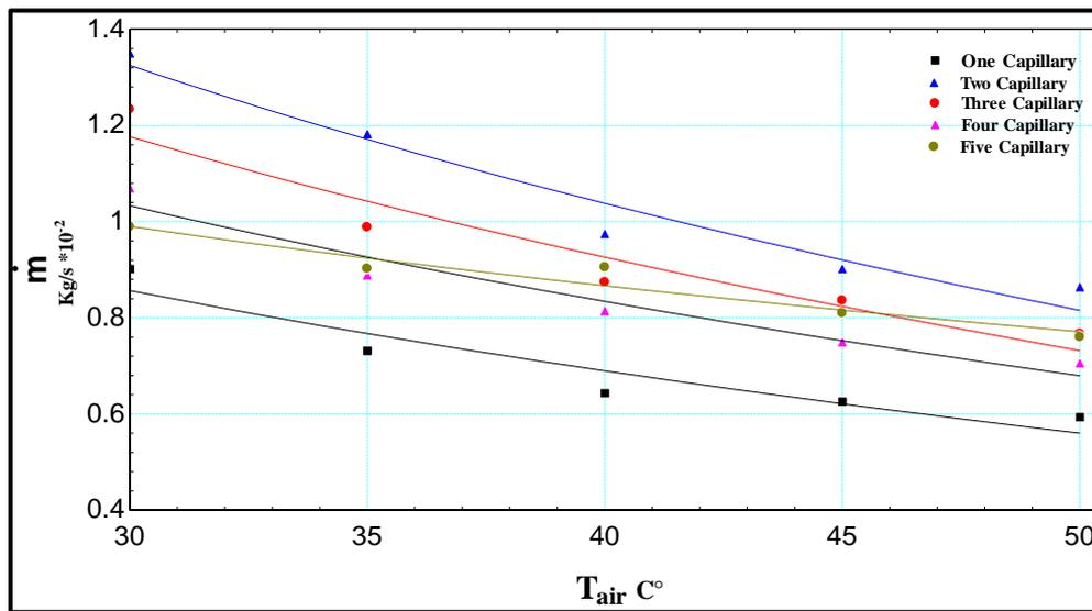
Figure (9) Refrigerant mass flow rate vs. ambient air temperature
