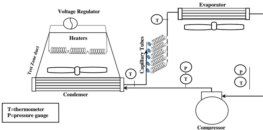
Figure (2) Sketch of test rig with measuring devices
