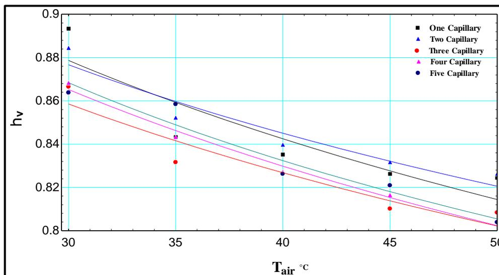
Figure (10) Compressor volumetric efficiency vs. ambient air temperature
