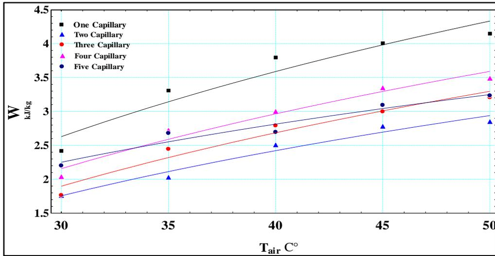
Figure (3) Compressor work vs. capillary tube number
