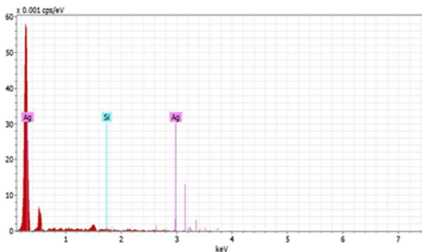
Figure (7): Shows the EDX chart of Ag NPs on silicon substrate
