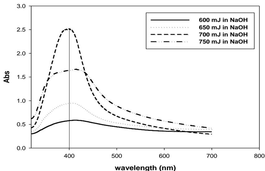
**Figure (3): Absorbance spectrum of AgNPs for different values of the energy of the laser beam**
