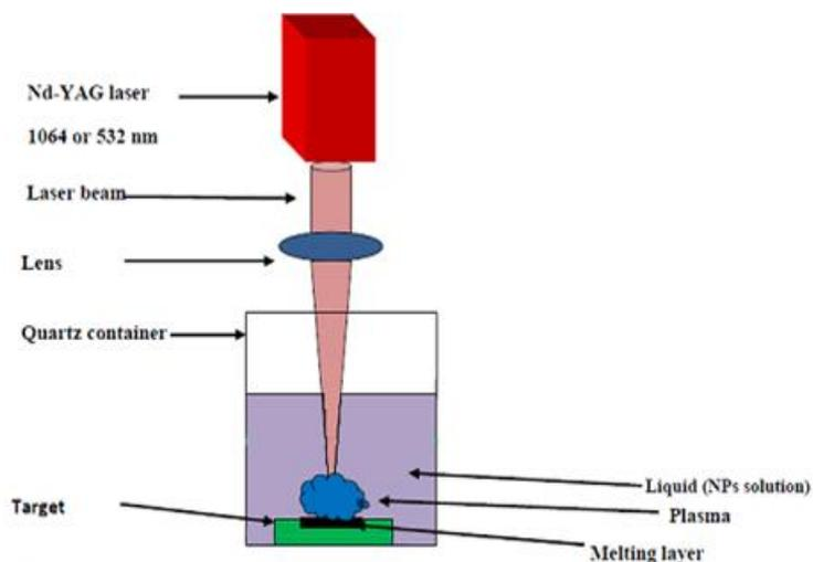
**Figure (1) Experimental setup for nanoparticles synthesis, by laser ablation technique[1]**
