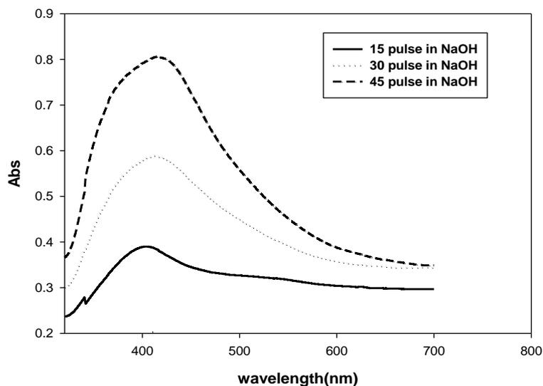
**Figure (2): Absorbance spectrum of AgNPs for different values of number of pulses**
