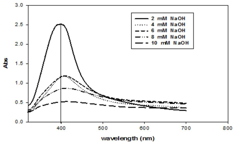
Figure (5): Absorbance spectrum of AgNPs for different values of the NaOH concentrations
