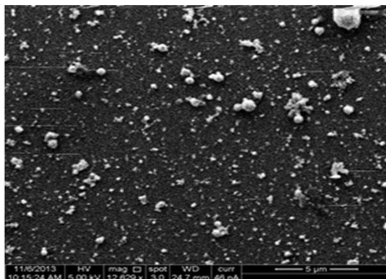
Figure (6): Shows the SEM image of Ag NP on silicon substrate
