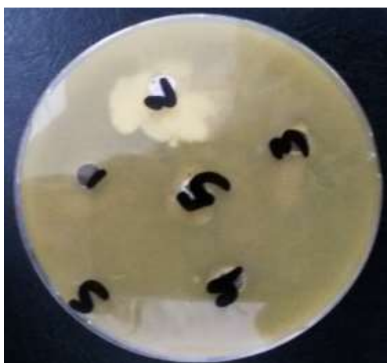
Figure 12 anti-bacterial activity for MgO after 24 hr: 1) TiO 2 sample, 2)MgO sample, 3)MgO+2% TiO 2 sample, 4)MgO+5%TiO 2 , sample 5)MgO+10%TiO 2 sample
