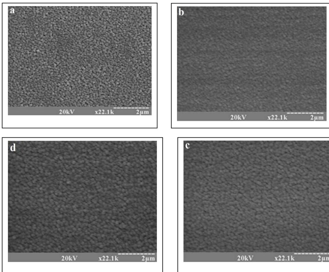
**Fig. 4: SEM Image for CdSe Thin Film at different ratio**
