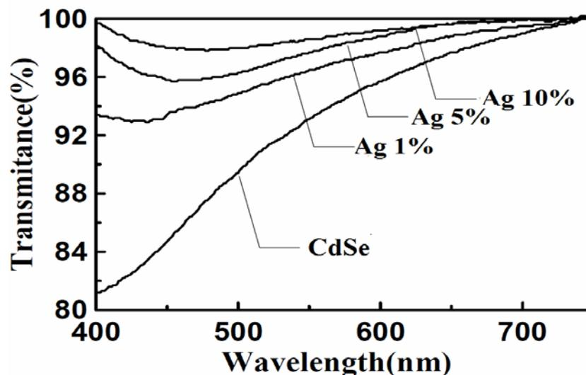
Fig.1: Transmittance spectra of CdSe Thin Films Deposited at different Ratio
