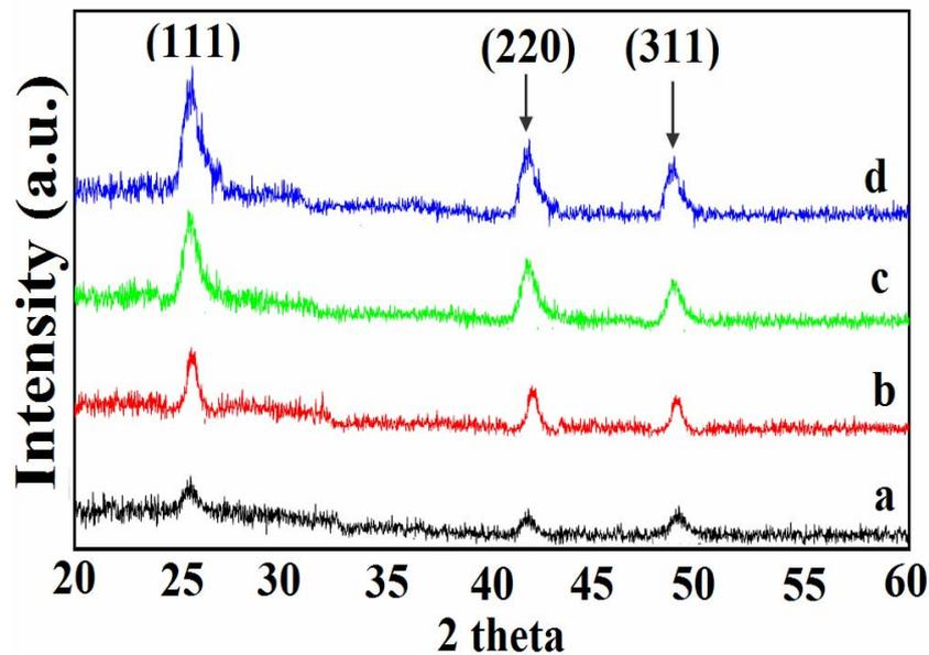
Fig. 3: XRD Patterns of CdSe Thin Films at different ratio
