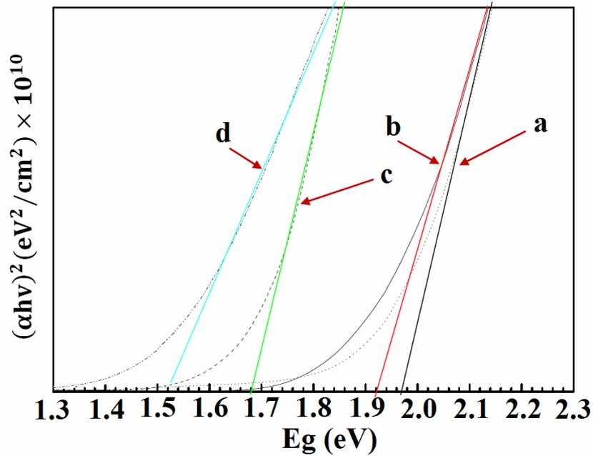
Fig. 2: Plot of  $(\alpha h\nu)^2$  versus  $E_g(\text{eV})$  of CdSe Thin Film of different ratio
