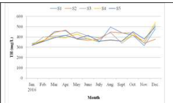
Figure 13- Variation of the total hardness values on the Dejjala River during the study period
