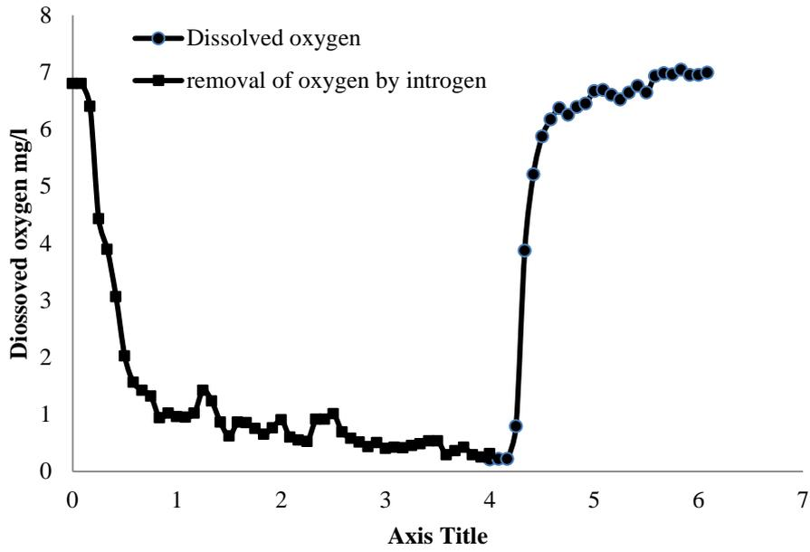
Figure 4. Dissolution and removal of oxygen in the distilled water.
