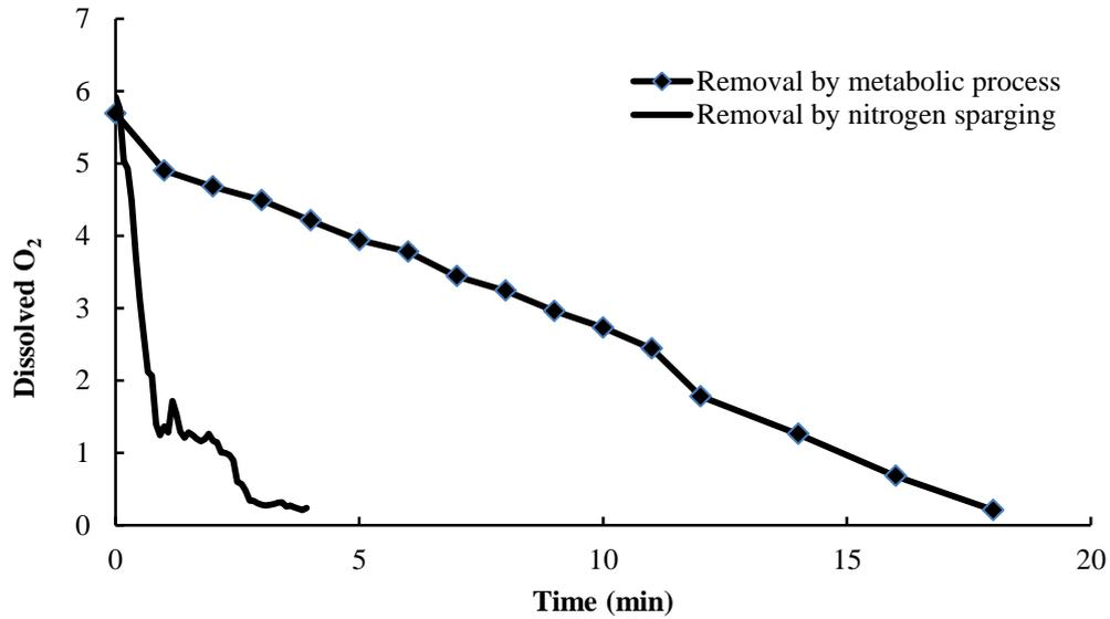
Figure 6. Dissolved oxygen in the distilled water, when the bioreactor removed by pure nitrogen, as well as in wastewater when the removal carried out by a metabolic process.
