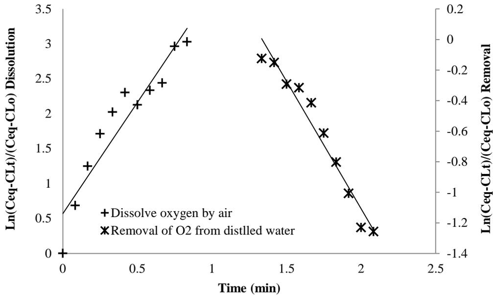
Figure 5. Volumetric mass transfer coefficient in dissolution and removal process with distilled water.
