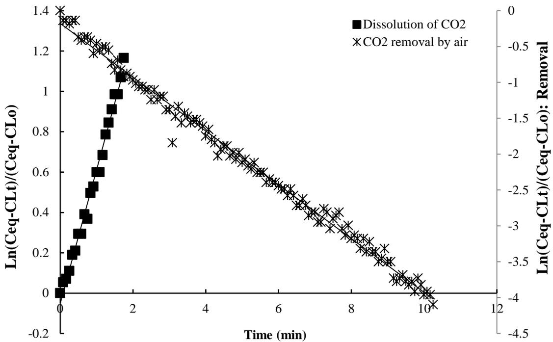
Figure 7. Volumetric mass transfer coefficient in dissolution and removal process with distilled water.
