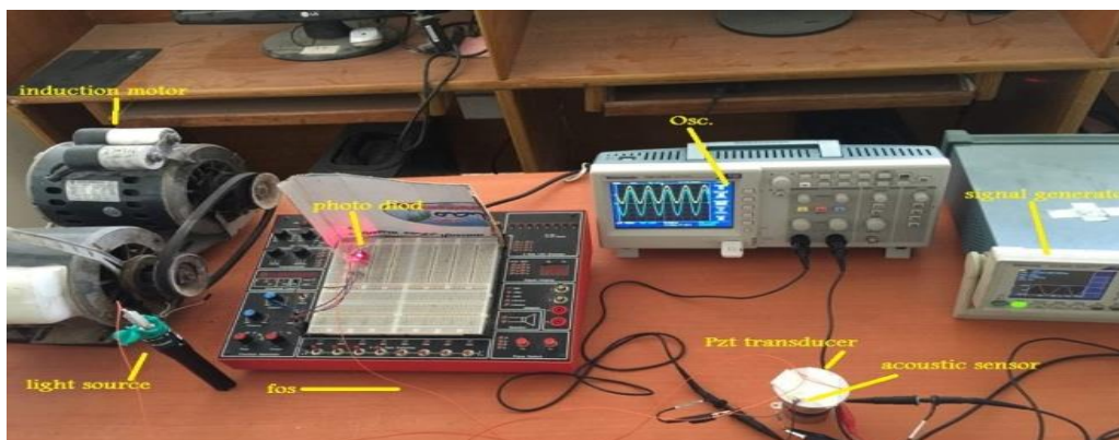
Figure 4: System used to measure vibrations of induction motor using piezoelectric sensor
