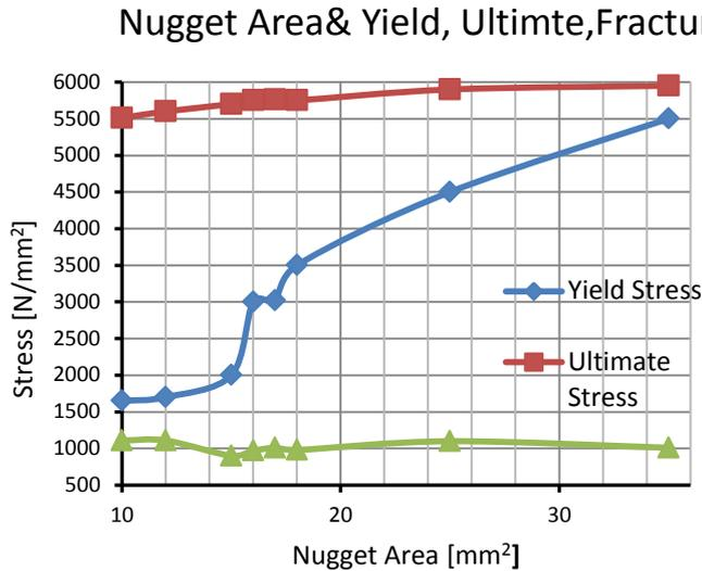
Figure 7: Relationship between Nugget area and stress under tensile test for first group samples
