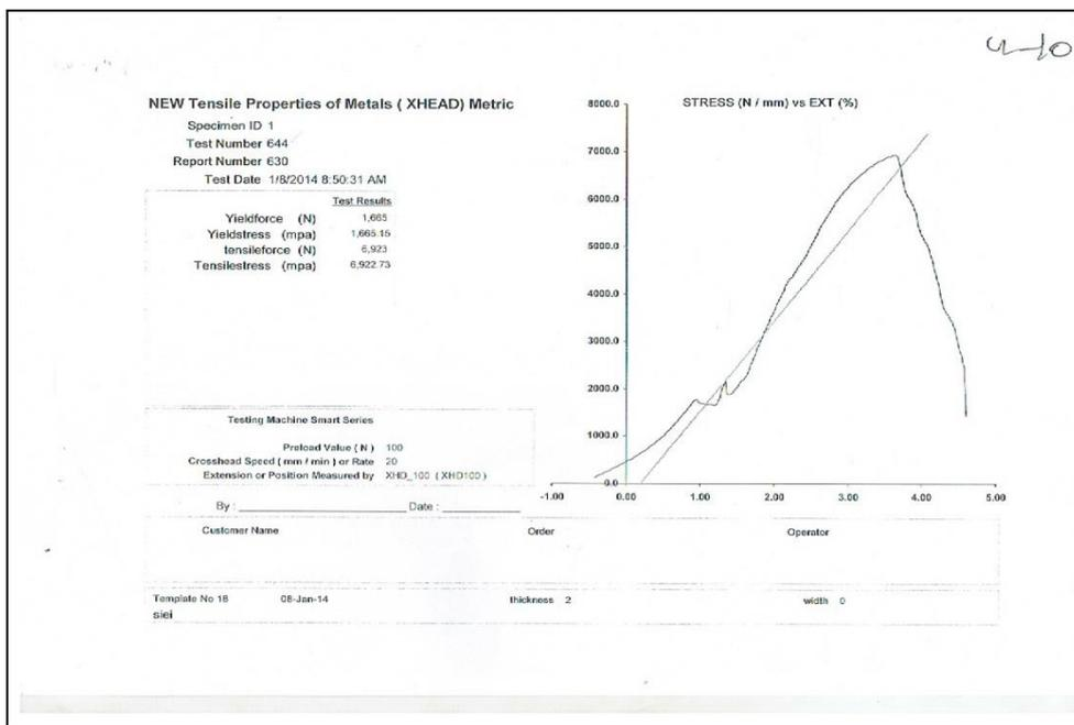
Figure 6: Tensile test for second group of the samples.
