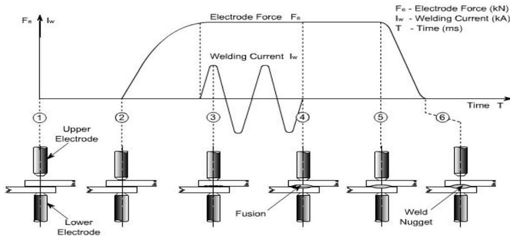
Figure 1: Resistance spot welding cycle [13]
