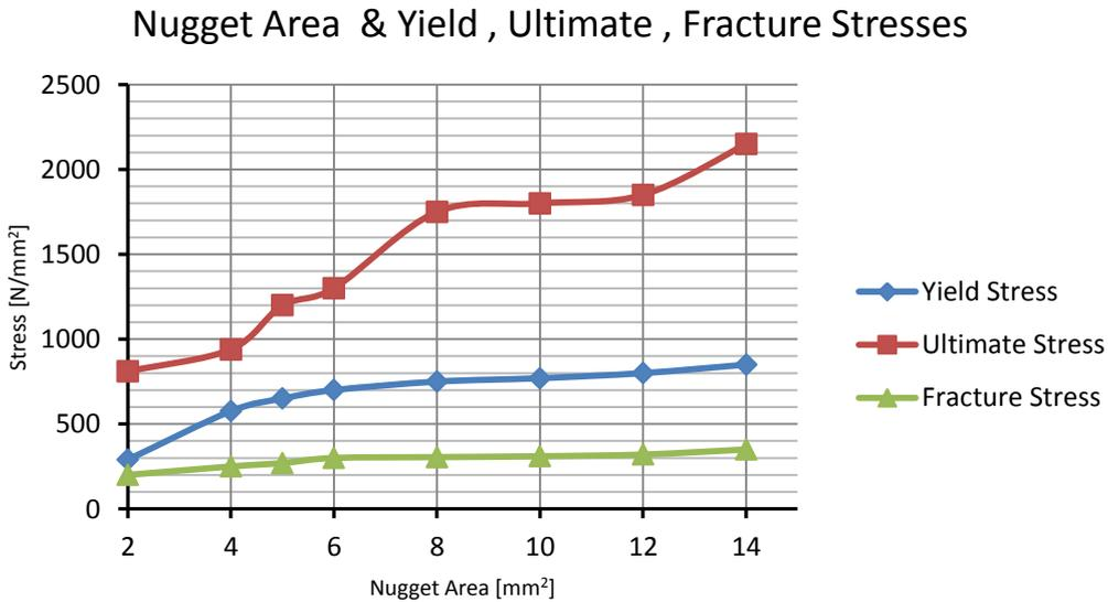
Figure 8: Relationship between Nugget area and stress of spot welding under tensile test for second group samples considering the effect of applying force.
