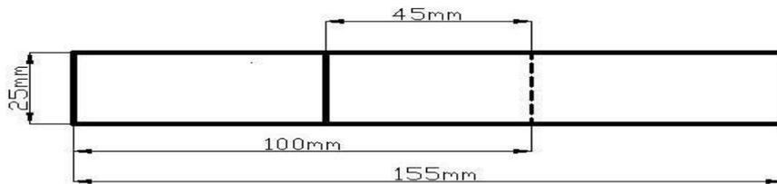
Figure 2: Dimensions of specimen
