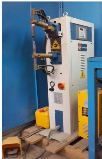
Figure 3: Pedestal-type spot welding machine
