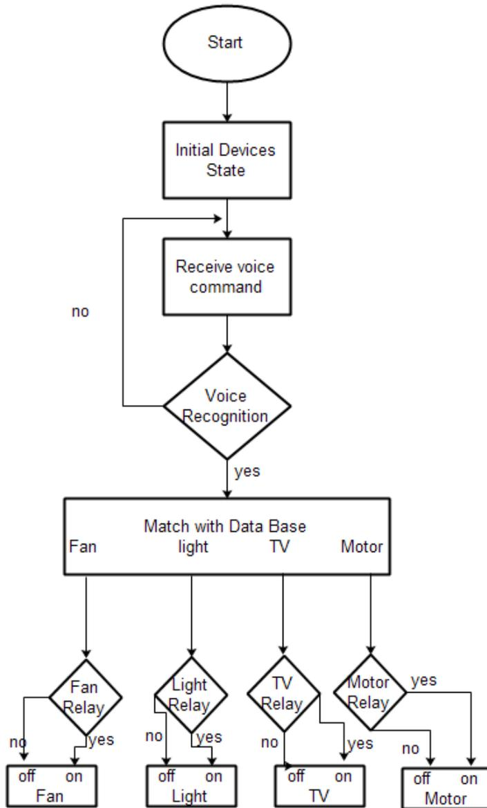
Figure (11): Flowchart for system algorithm
