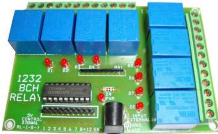
**Figure (6): Relay Board – 8 Channels**
