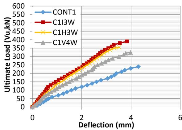
Figure 4: Load-Deflection Curve of Specimens in Group 3 (C1H3W, C1I3W and C1V4W)
