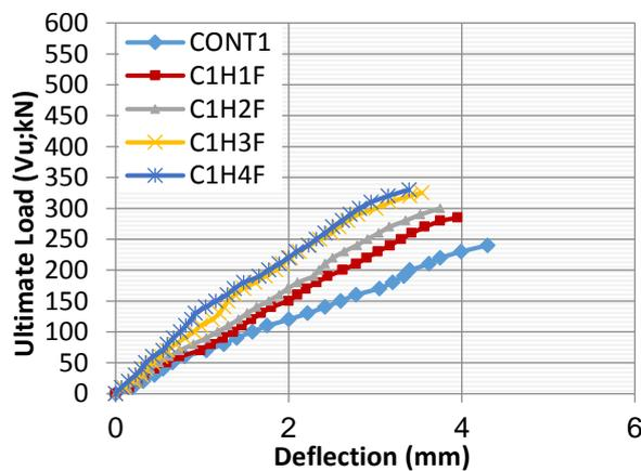
**Figure 2: Load-Deflection Curve of Specimens in Group 1 (C<sub>1</sub>H<sub>1</sub>F, C<sub>1</sub>H<sub>2</sub>F, C<sub>1</sub>H<sub>3</sub>F, and C<sub>1</sub>H<sub>4</sub>F)**
