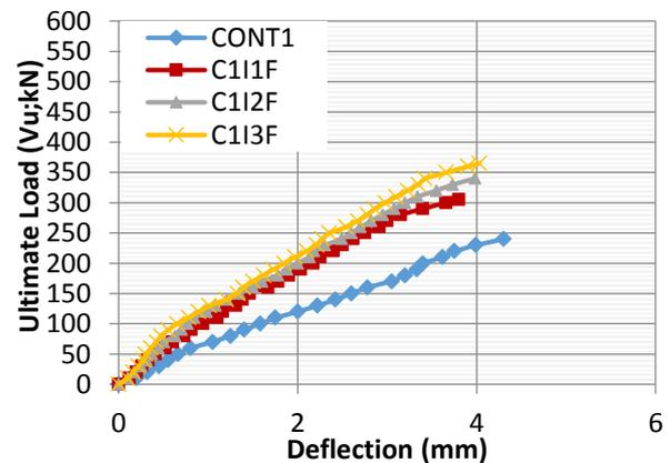
**Figure 3: Load-Deflection Curve of Specimens in Group 2 (C<sub>1</sub>I<sub>1</sub>F, C<sub>1</sub>I<sub>2</sub>F and C<sub>1</sub>I<sub>3</sub>F)**
