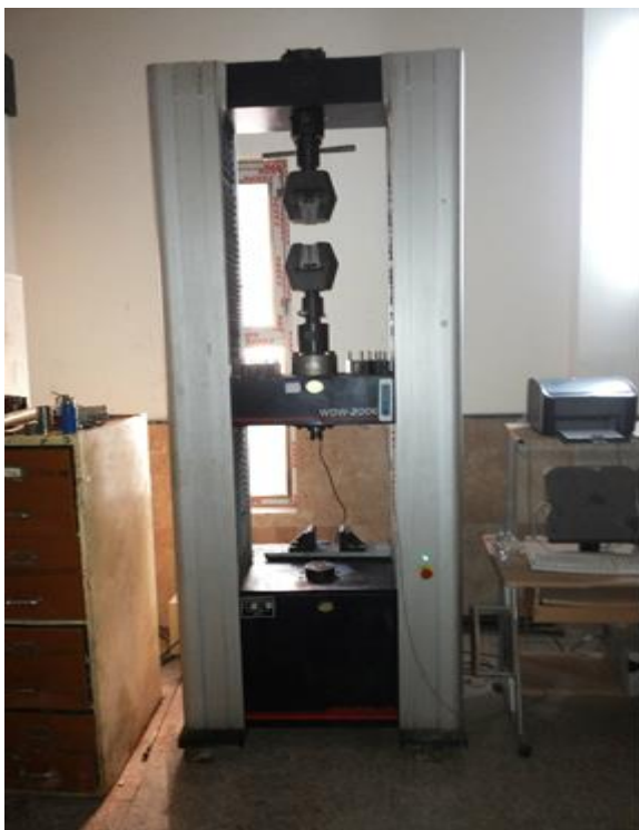
Figure 15: Tensile test machine type (WDW-200E)
