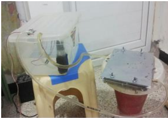
Figure 9: Feeding water pump
