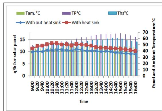
Figure 12. Solar panel efficiency in case of with and without heat sink and the temperatures of plane panel ( $T_p$ ), panel with heat sink ( $T_{hs}$ ) and ambient ( $T_{am}$ ) vs. time.
