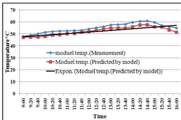
Figure 7: The temperature of module with heat sink as predicted and measured vs. time
