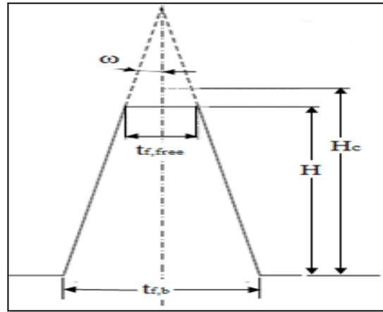
**Figure 2: The profile of trapezoidal fin**
