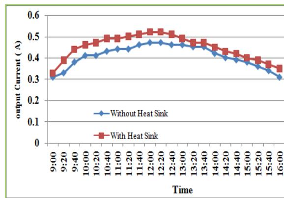
Figure 9: Solar panel output current with and without heat sink.
