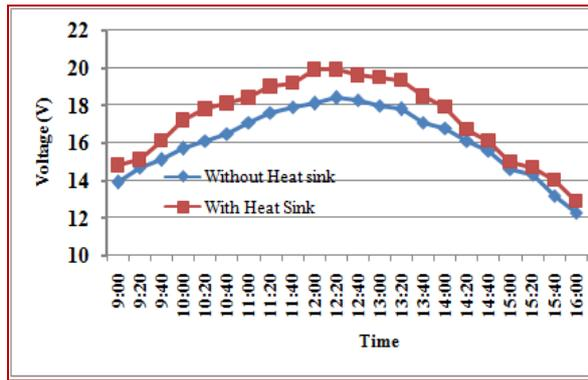
Figure 10: Solar panel output voltage without and with heat sink.
