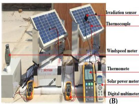
Figure 4: (A) Rear sides of the PV panels with and without heat sink, (B) Experimental set.
