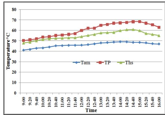
Figure 8: Ambient and different cases panel temperatures vs. time
