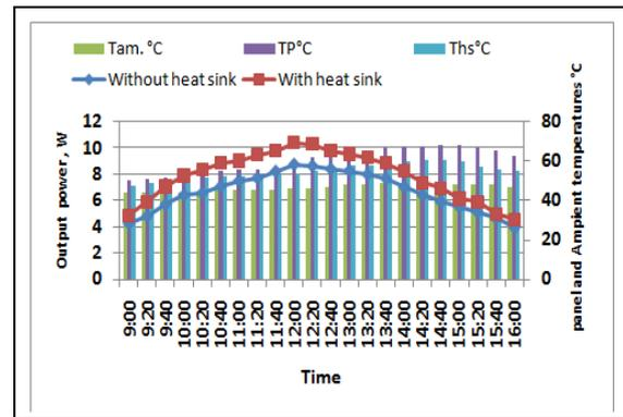
Figure 11. Solar panel output power in case of with and without heat sink and the temperatures of plane panel ( $T_p$ ), panel with heat sink ( $T_{hs}$ ) and ambient ( $T_{am}$ ) vs. time.
