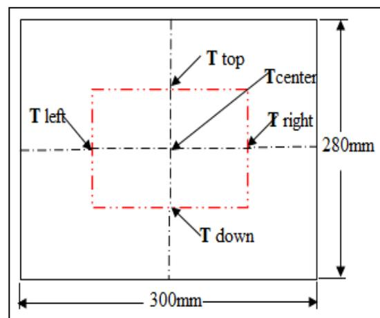
Figure 5: The locations of Temperature sensors
