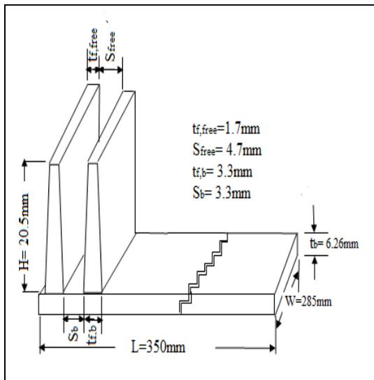
**Figure 1: Heat sink parameters**
