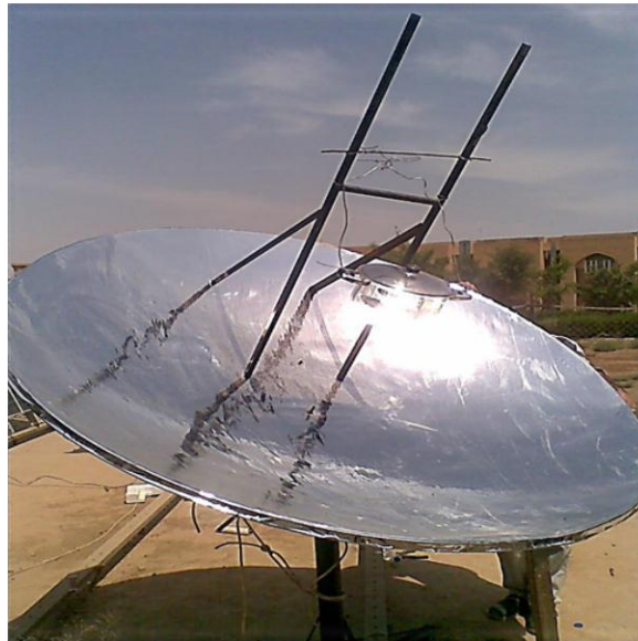
Fig. 1: Parabolic solar cooker used in the experiment.
