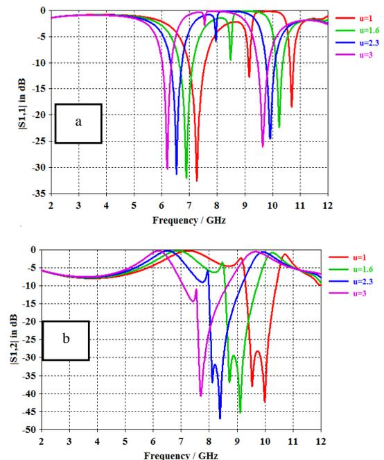
Figure 5: Parametric study of the proposed filter with  $u$  as a parameter: (a) Input reflection coefficient (S11), and (b) Insertion loss (S12)
