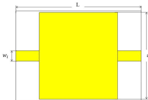
Figure 1: CST MWS model for the proposed BPF (top layer)
