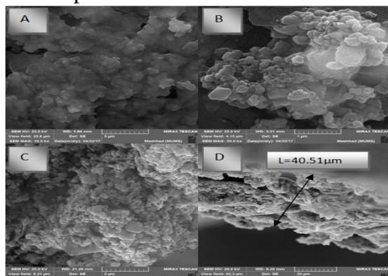
Figure 2. FESEM images of (A) ZnO without annealing, (B) ZnO annealed at 140 °C for 12 h, (C) ZnO -Ag
