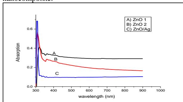
Figure 3. UV-Vis absorption spectra: A) ZnO Nps without annealing, B) ZnO NPs annealed at 140 °C for 12 h, C) ZnO -Ag nanocomposite.
