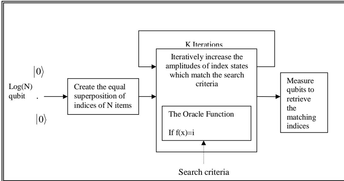
**Figure (1) the block diagram of Grover's algorithm**
