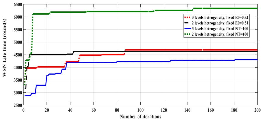
Fig. (8) Network life time vs. PSO algorithm iterations
