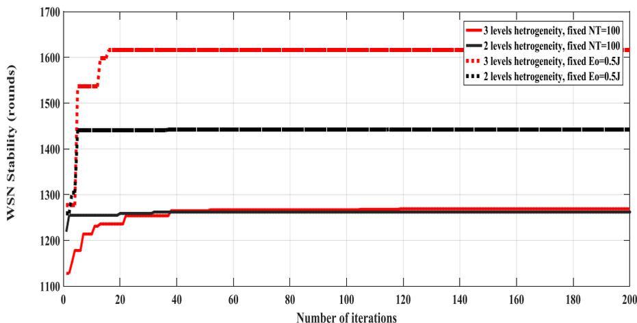
Fig. (7) Network stability vs. PSO algorithm iterations
