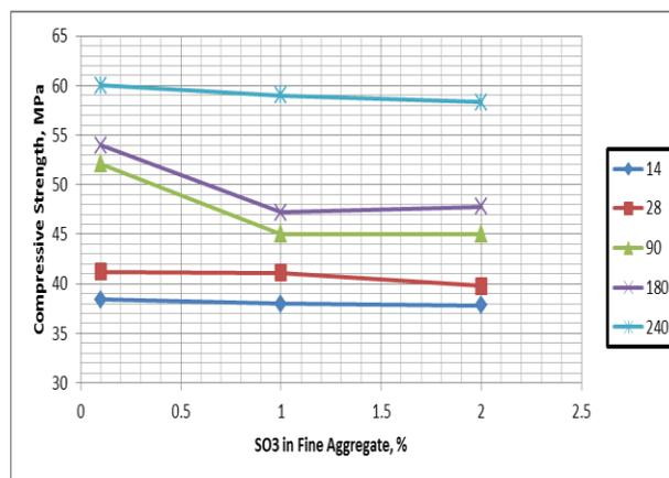
**Figure 2: The effect of  $\text{SO}_3$  content in fine aggregate on the development of compressive strength through days (14, 28, 90, 180, and 240 day) for mixes R60, R60S1 and R60S2**
