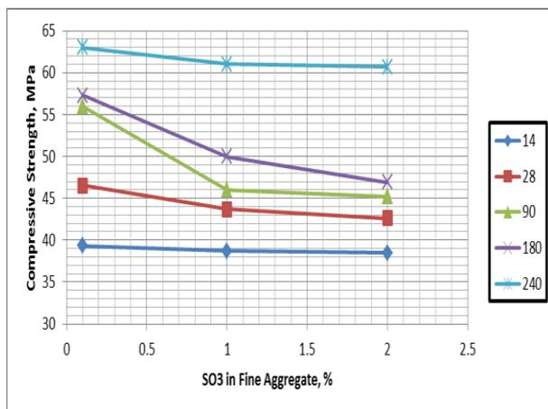
**Figure 1: The effect of  $\text{SO}_3$  content in fine aggregate on the development of compressive strength through days (14, 28, 90, 180, and 240 day) for mixes R50, R50S1 and R50S2.**
