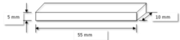
Figure 1: Impact test specimen [5]
