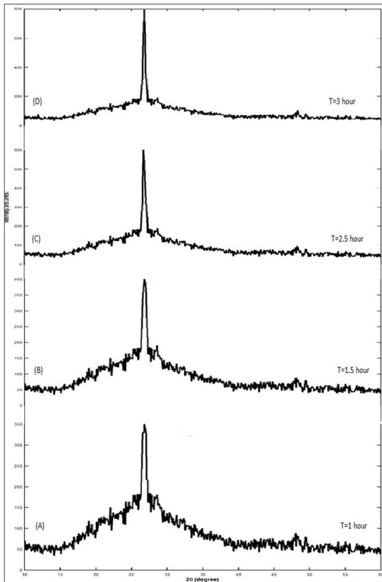
Figure 2: XRD pattern of hexagonal structure CdS thin film at (A) 1 hour (B) 1.5 hour (C) 2.5 hour (D) 3 hour with ( $P=2 \times 10^{-2}$  mbar,  $V=2$  K $v$ )
