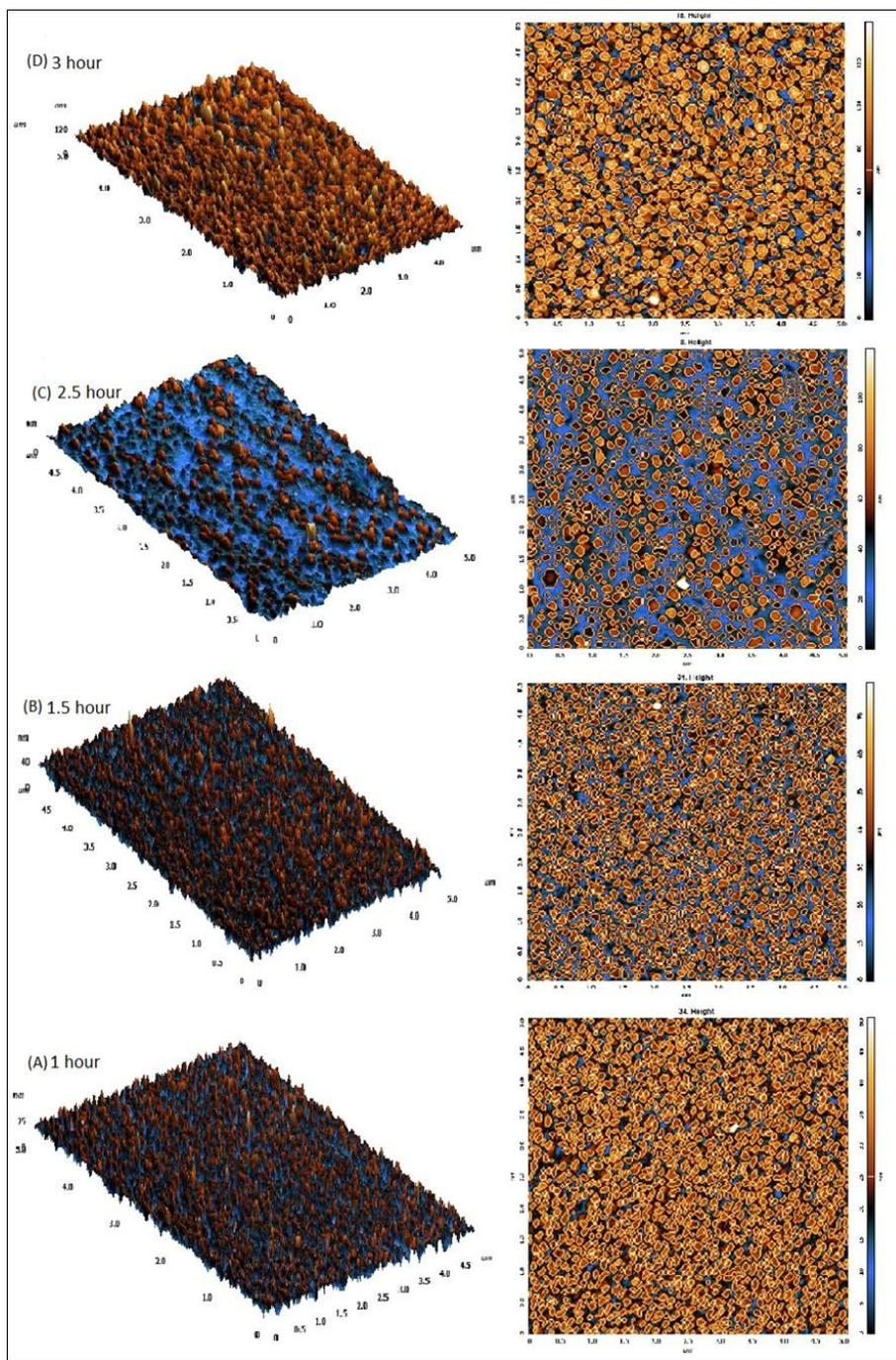
Figure 4: AFM images of CdS thin film at (A) 1 hour (B) 1.5 hour (C) 2.5 hour (D) 3 hour with ( $P=2 \times 10^{-2}$  mbar,  $V=2$  Kv)
