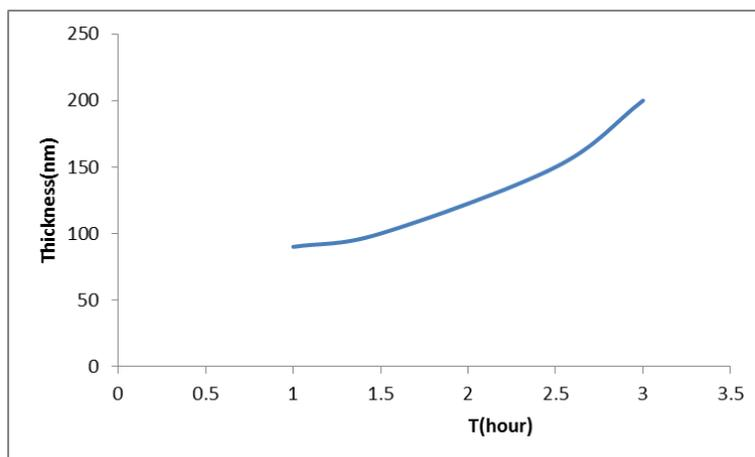
Figure 1: The variation of the films thickness as a function of sputtering time
