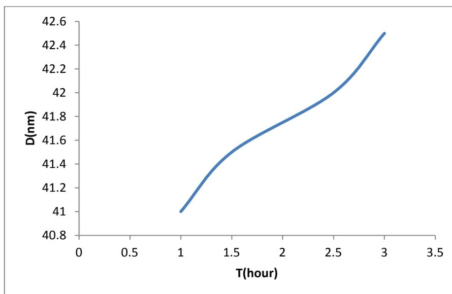
Figure 3: The variation of the grain size as a function of sputtering time
