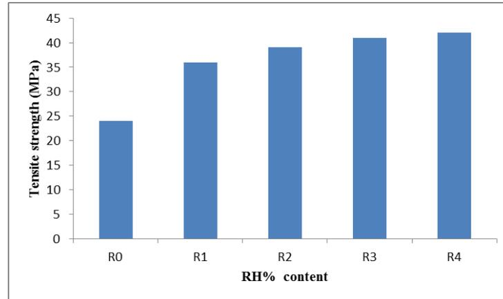
**Figure 3. Tensile strength values for the prepared composite**
