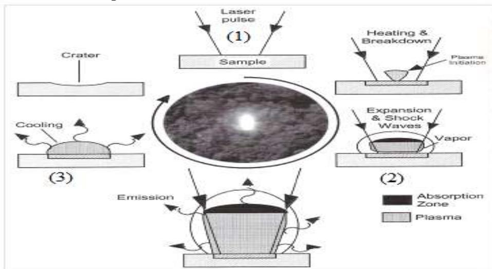
**Figure 1**-Life cycle diagram showing of the main events in the LIBS process [4].
