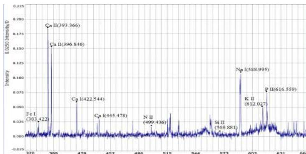
**Figure 7**-LIBS spectra recorded from Fallujah soil.
