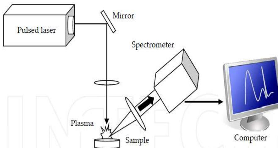
**Figure 3-**A schematic diagram of the LIBS system.
