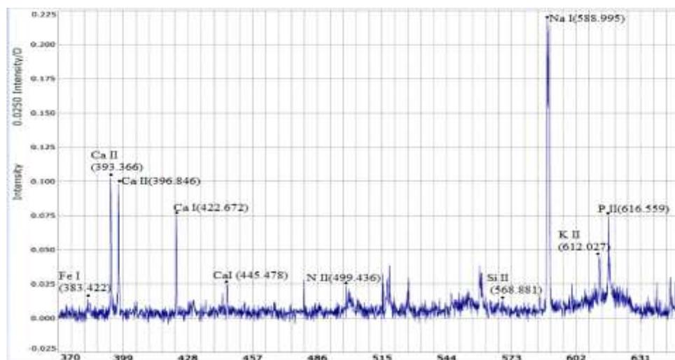
**Figure 6**-LIBS spectra recorded from Garmah soil.
