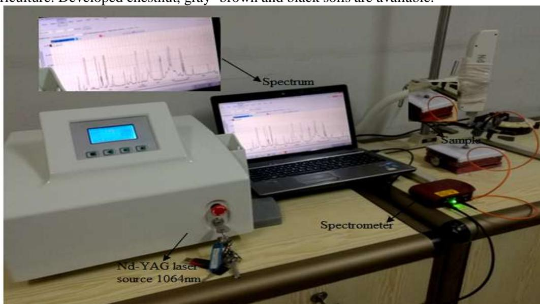
**Figure 2-**Laser-induced breakdown spectroscopy system
