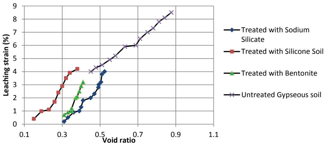
Figure 4. Leaching strain-void ratio relation for treated and untreated gypseous soil
