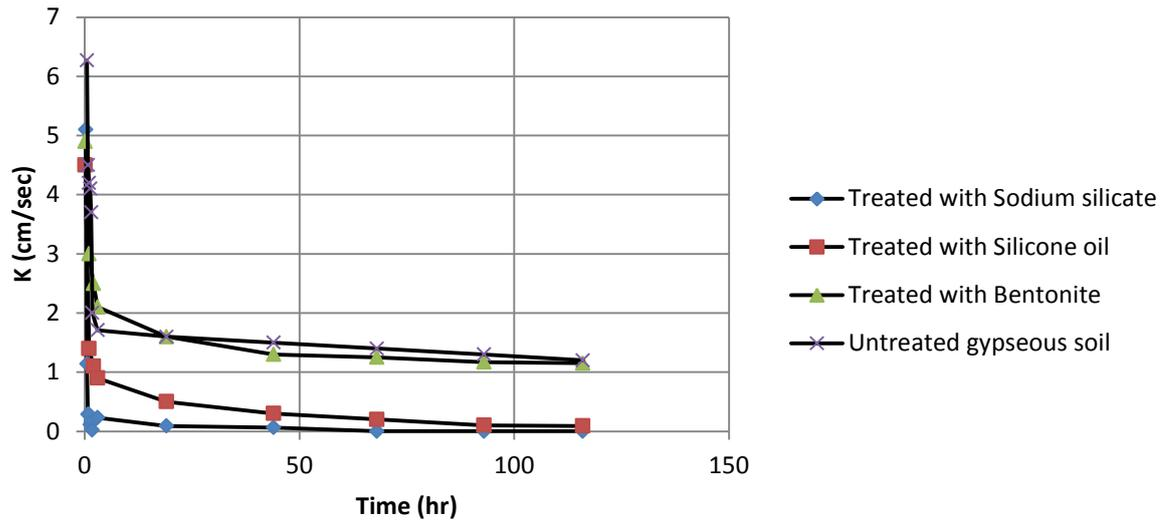
Figure 8. Coefficient of permeability-time relation for treated and untreated gypseous soil.
