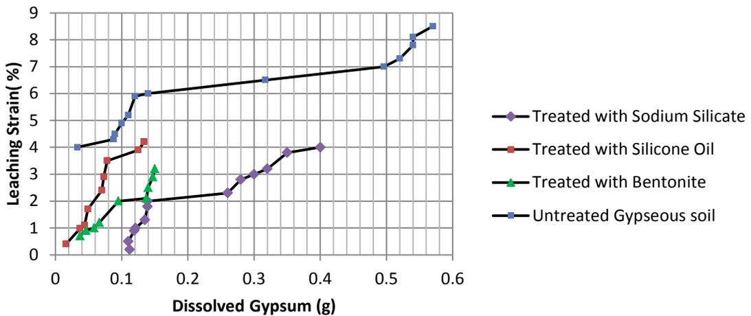
Figure (3).Leaching strain–dissolved gypsum relation for treated and untreated gypseoussoil.
