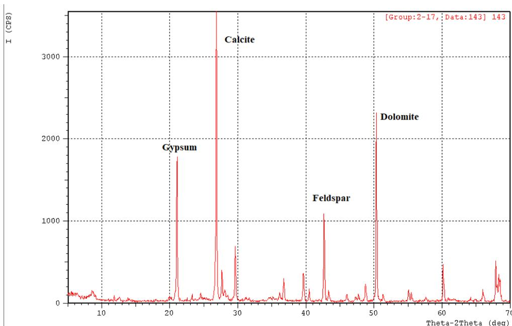
Figure 2. XRD for gypsum rich soil.
