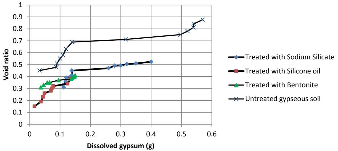
Figure 5. Void ratio-dissolved gypsum relation for treated and untreated gypseous soil.
