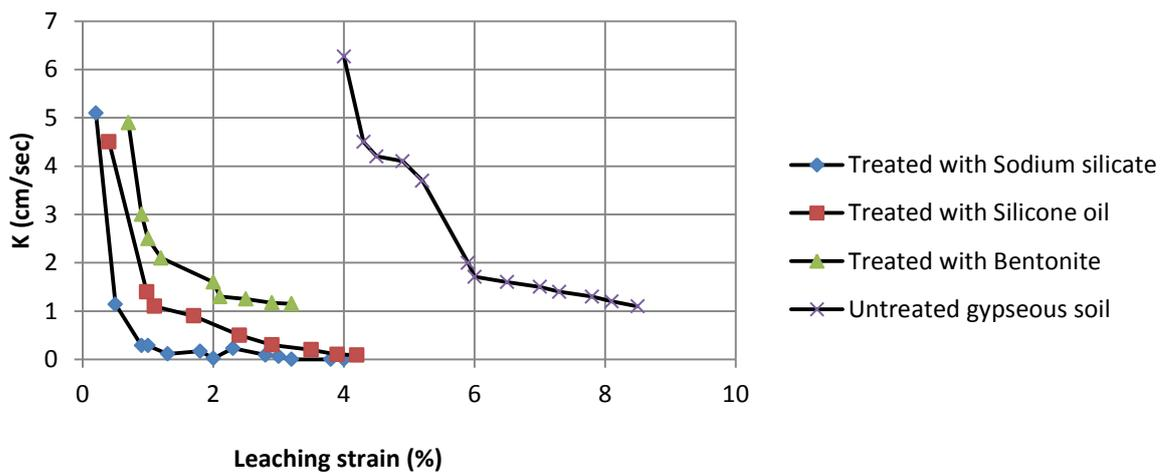
Figure 7. Coefficient of permeability-leaching strain relation for treated and untreated gypseous soil.
