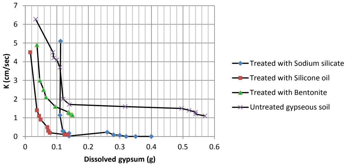
Figure 6. Coefficient of permeability-dissolved gypsum relation for treated and untreated gypseous soil.
