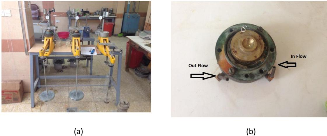
Figure 1. a) Oedometer-permeability leaching apparatus, b) Leaching oedometer cell.
