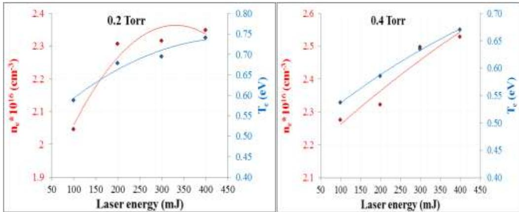
**Figure 6-** The difference of ( $T_e$ ) and ( $n_e$ ) against the laser energies for a Copper target in without magnetic field
