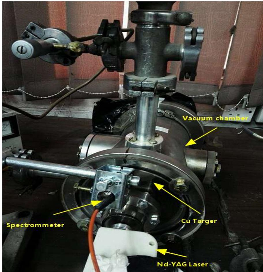
Figure1- the experimental set up of LIBS system
