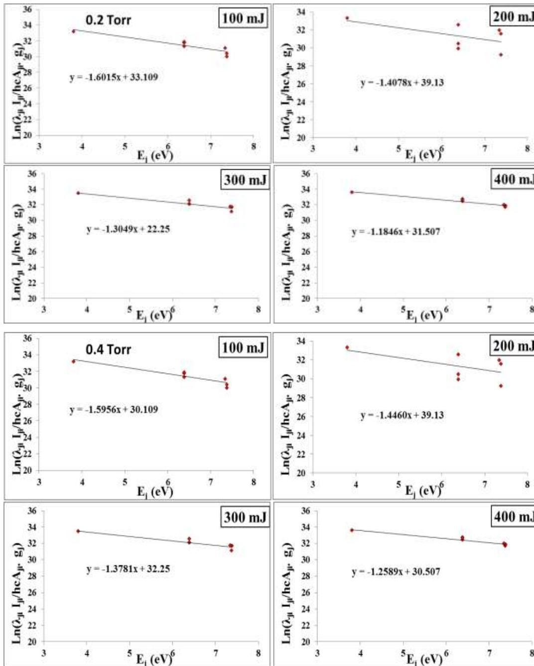
Figure 3- Boltzmann plot for a copper target with existence magnetic field.
