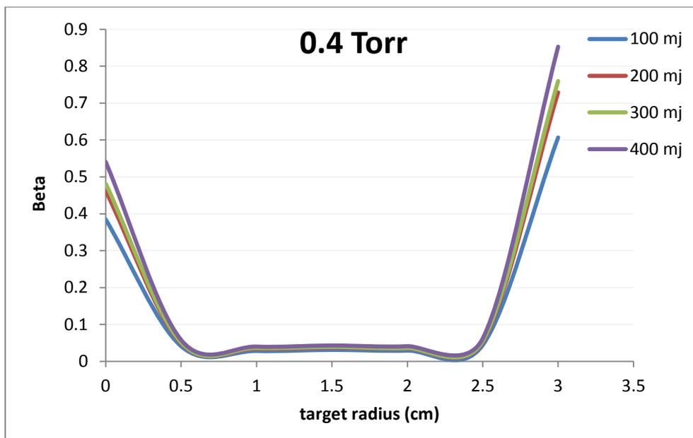
Figure 8- The different beta with the target radius for a Copper target in 0.4 Torr
