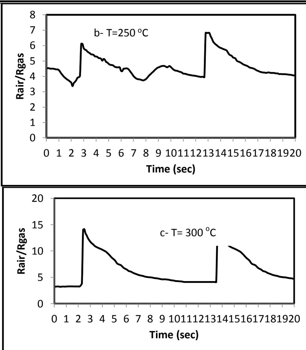
Figure (3): The gas sensor (of  $t_1=102.69$  nm) response at 6 volt bias voltage and operating temperature ((a) 200, 250 (b) and 300 (c)) °C.
