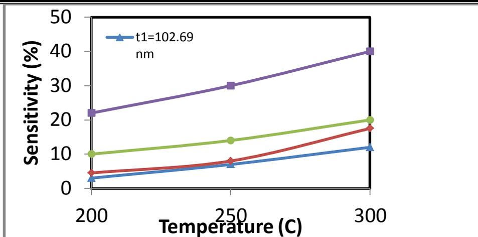
Figure (4): the sensitivity variation with operating temperature for each sample thickness
