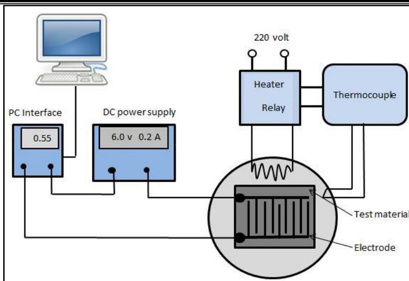
Figure (2): scheme of the used gas sensor testing setup.
