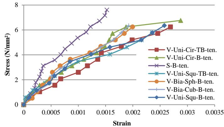
Figure 8. Stress-strain relationships (tension)
