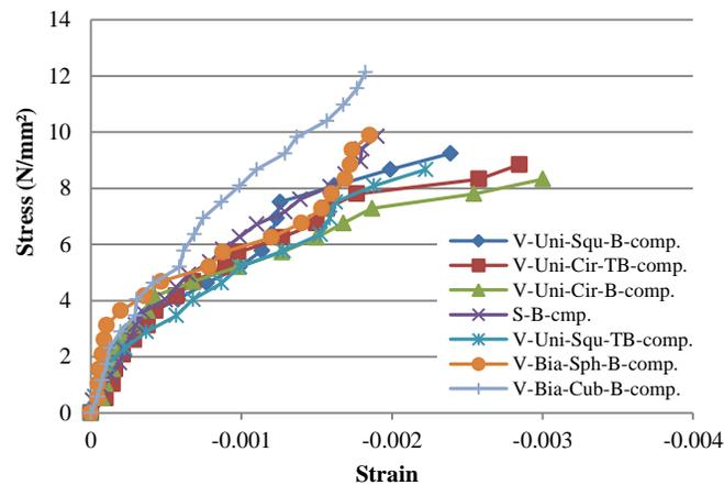
Figure 9. Stress-strain relationships (compression).
