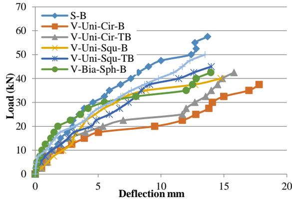
Figure 4. Load - mid span deflection curves of all specimens
