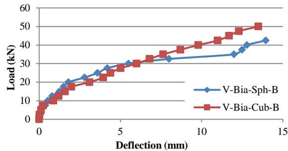
Figure 6. Load - mid span deflection curves of specimens with biaxial voids.
