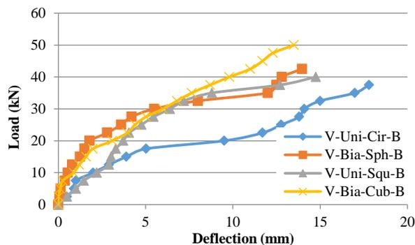
Figure 7. Load - mid span deflection curves of specimens with biaxial and uniaxial voids
