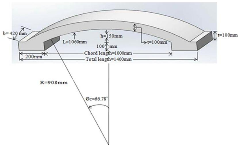
Figure 1. Geometry of the cylindrical shell model
