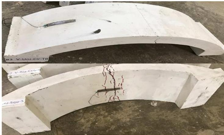
Figure 10. Crack Patterns of (V-Uni-Cir-TB)
