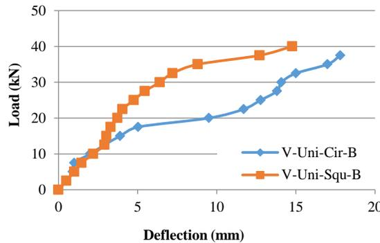
Figure 5. Load - mid span deflection curves of specimens with uniaxial voids.
