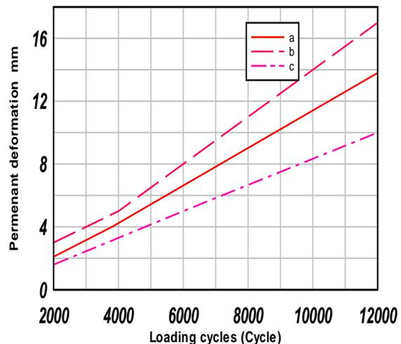
Fig 4 Hamburg Wheel – Track Testing, a) reference asphalt, b) RAP A, c) RAP B.
