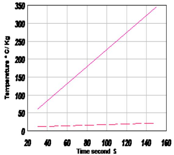
Fig 2 Temperature change by microw-ave of a) Aggregate with Sand, continu-ous line. B) Bitumen, dashed line.
