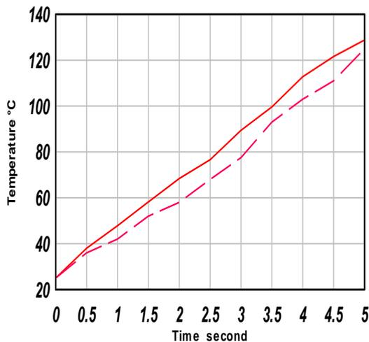
Fig 3 The increasing of temperature with time exposure of microwave radiation a) dashed line for samples B; b) continues line for (RAP) B samples.
