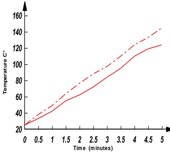
Fig 1 The increasing of temperature with time of exposure by microwave, a) continuous line samples A, b) dashed line for RAP A.
