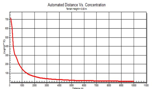
Figure 9: SO2 dispersion for the L1 unit
