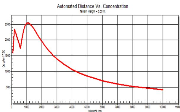
Figure 5: SO2 dispersion for the R2 unit
