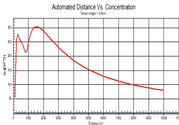
Figure 14: SO2 dispersion for the C2 unit.
