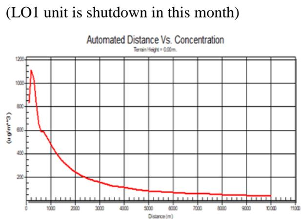
Figure 23: SO2 dispersion for the P2 unit
