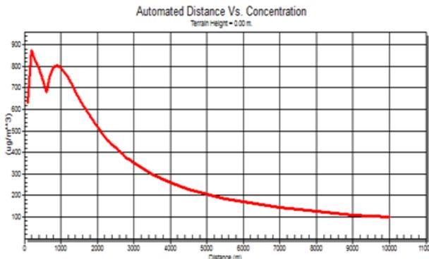
Figure 3: SO2 dispersion for the R1 unit
