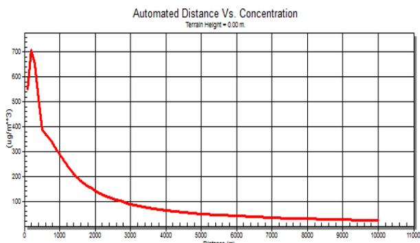
Figure 10: SO2 dispersion for the L2 unit.
