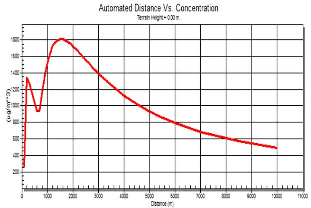
Figure 6: SO2 dispersion for the C13 unit.
