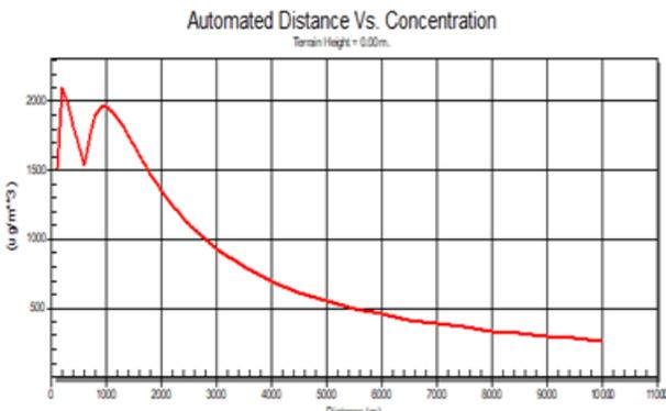
Figure 17: SO2 dispersion for the R2 unit
