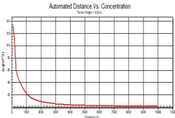
Figure 18: SO2 dispersion for the C13 unit
