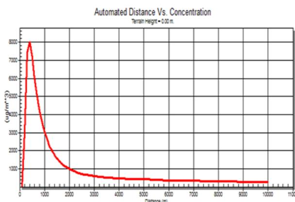
Figure 26: Illustrates the stability C (Slightly unstable)
