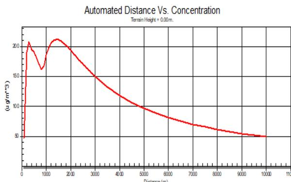
Figure 13: SO2 dispersion for the C1 unit.
