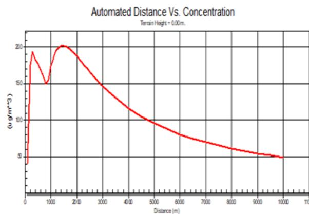
Figure 1: SO2 dispersion for the C1 unit
