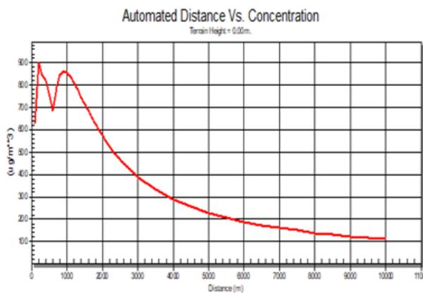
Figure 15: SO2 dispersion for the R1 unit
