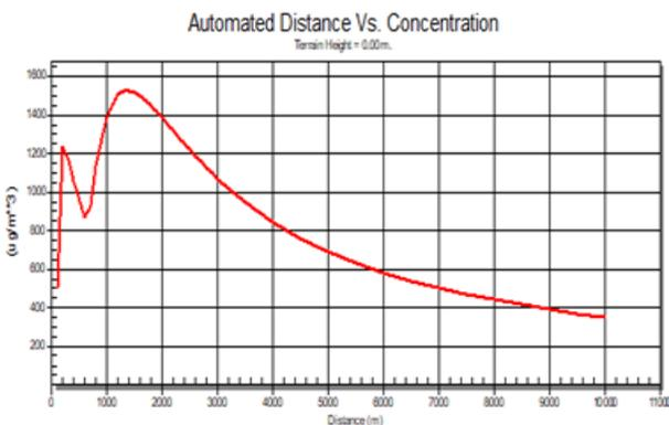
Figure 19: SO2 dispersion for the P1 unit
