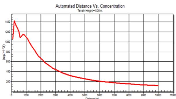
Figure 11: SO2 dispersion for the L3 unit.
