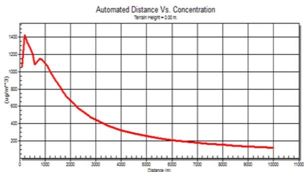
Figure 12: SO2 dispersion for the P2 unit
