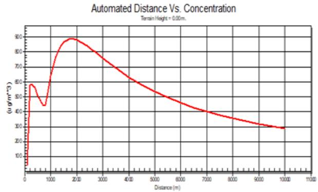
Figure 20: SO2 dispersion for the P3 unit
