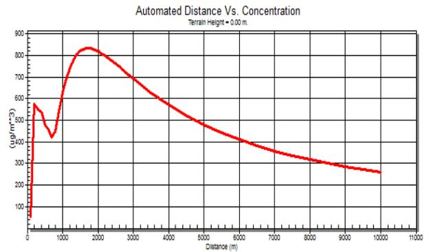
Figure 7: SO2 dispersion for the P1 unit
