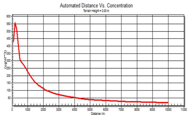
Figure 8: SO2 dispersion for the P3 unit.
