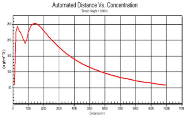
Figure 2: SO2 dispersion for the C2 unit
