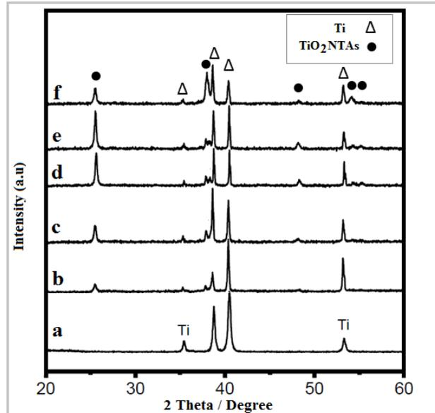
Figure 1: XRD patterns showing the (a) Ti foil and different stages of TiO<sub>2</sub> NTAs film formation at 40 V in NH<sub>4</sub>F/EG/H<sub>2</sub>O solution for (b) 1 min (c) 15 min (d) 30 min (e) 60 min and (f) 120 min.
