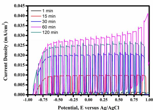
Figure 4: photocurrent responses of TiO<sub>2</sub> NTAs prepared at different anodization duration
