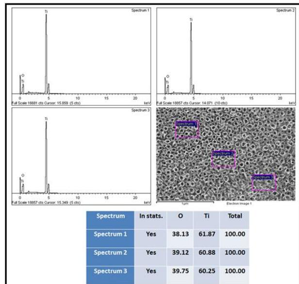
Figure 3: EDX spectra of TiO<sub>2</sub> NTAs prepared at 60 min anodization duration.
