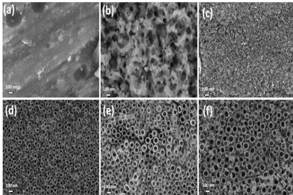
Figure 1: FESEM images showing the (a) Ti foil and different stages of TiO<sub>2</sub> NTAs film formation at 40 V in NH<sub>4</sub>F/EG/H<sub>2</sub>O solution for (b) 1 min (c) 15 min (d) 30 min (e) 60 min and (f) 120 min
