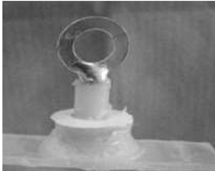
Figure (2): translucent plastic tube fixed with sticky wax and filled with composite with screw embedding in it.
