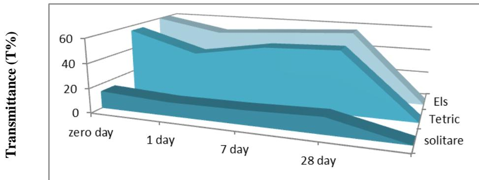
Figure(2): Histogram showing differences in transmittance percentage (T%) for different types of composite resin.
